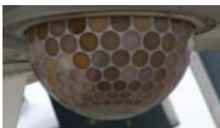
(left) Emitter array for internal SPS-171/172 electronically steerable jammer, dedesigned to focus jamming power into a narrow sector (podded L-005 depicted). (centre) Detector aperture for the MAK series infrared Missile Approach Warning System, here installed on a Bear H. (right) The ventral OBP-15T remote TV bombsight is used to target dumb bombs. The fairing for this device is well placed to fit a laser targeting system.
