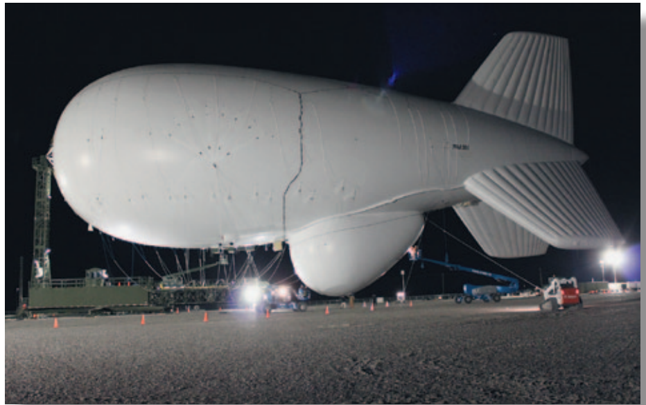
The long delayed JLENS tethered Over-The-Horizon radar was intended to provide US Army Patriot batteries, and US Navy warships defending beachheads, with an affordable capability to detect and attack cruise missiles. JLENS was cancelled in recent budgetary cuts.
