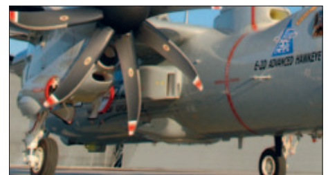
The circular ventral antenna on this E-2D belongs to the Cooperative Engagement Capability system, which permits the E-2D to function as an Over-The-Horizon targeting system for SAM shots.
