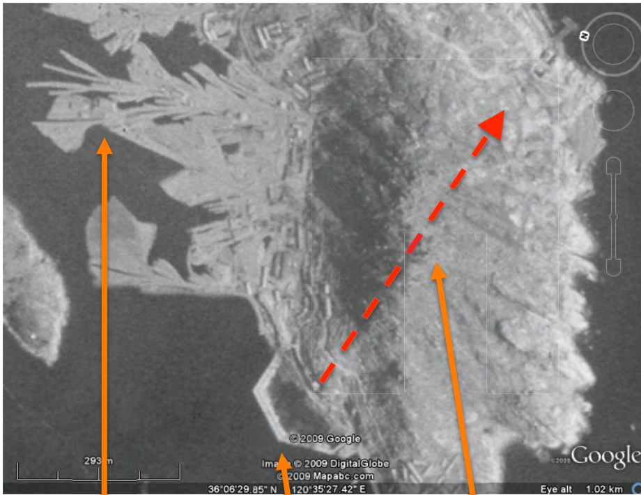
Tailings used as fill Coffer dam Tunnel dig Dock and base Tunnel entrance Residual drill, exit
