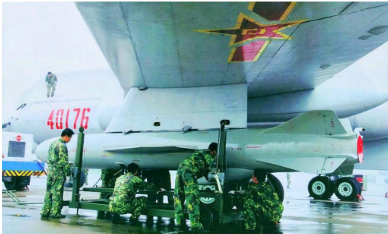
Figure 23: These images depict a H-6 Badger being armed with the KD-63, which is an indigenous PLA-AF cruise missile (PLA).
