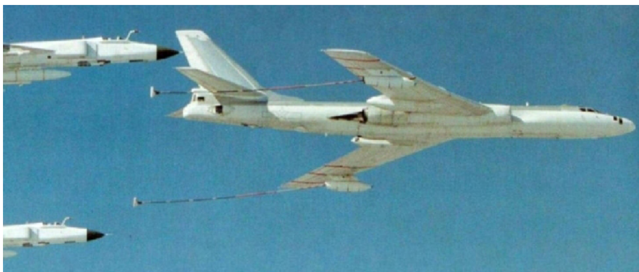
Figure 28: The Xian H-6 is the basis of China's indigenous aerial refuelling tanker program. Development was reported to be initially a collaboration with Flight Refuelling Limited in the UK during the 1980s. With the questionable usefulness of the Badger as a conventional strike aircraft, it is likely many more will be converted to tankers, especially given the low age of much of the Badger fleet. As a tanker the Badger compares closely to the now retired RAF Victor K.2 (PLA).
