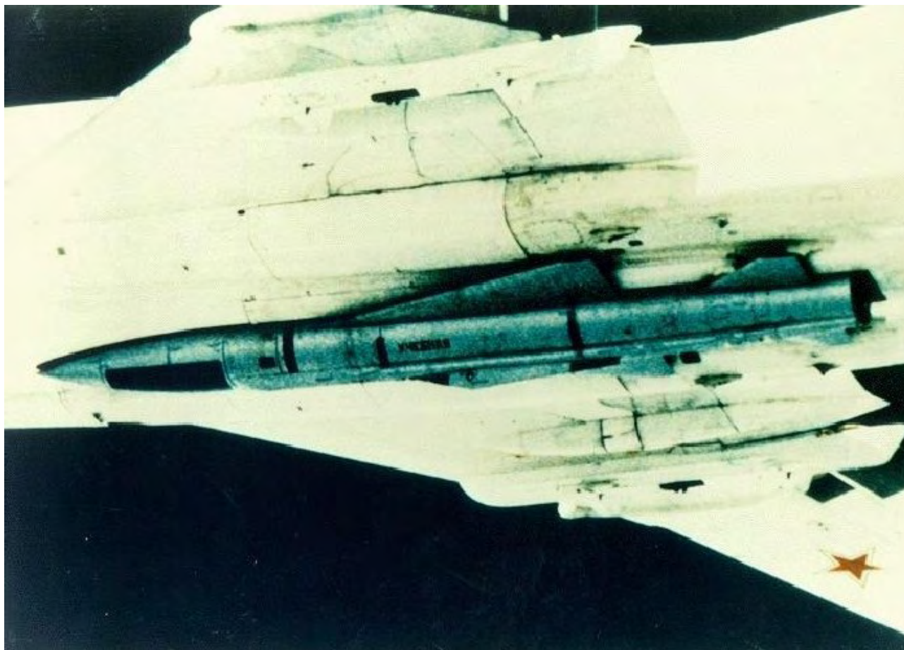
Figure 44: Kh-22M Burya. The Kh-22 series of supersonic cruise missiles was developed during the 1960s and is equivalent to the RAF's former Blue Steel missile carried by the V-bomber fleet. This Mach 3 missile is the primary weapon of the Tu-22M-3 Backfire C bomber, available in anti-shipping and land attack variants. Reports claim a mid life upgrade has been designed. As it employs identical liquid propellants to the PLA's Silkworm/Kraken, introduction of this missile presents no difficulties for the PLA (US DoD, RuMoD).
