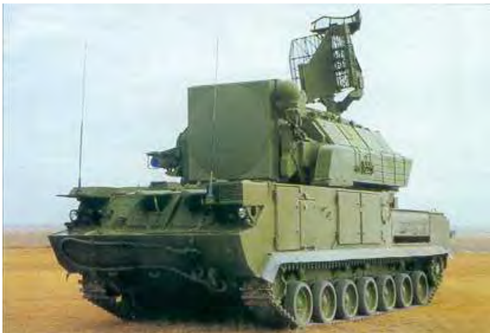
Figure 39: The PLA acquired several batteries of the Tor M1 (SA-15 Gauntlet) point defence SAM during the 1990s. With phased array capability, this system is difficult to jam (Rosoboronexport).
