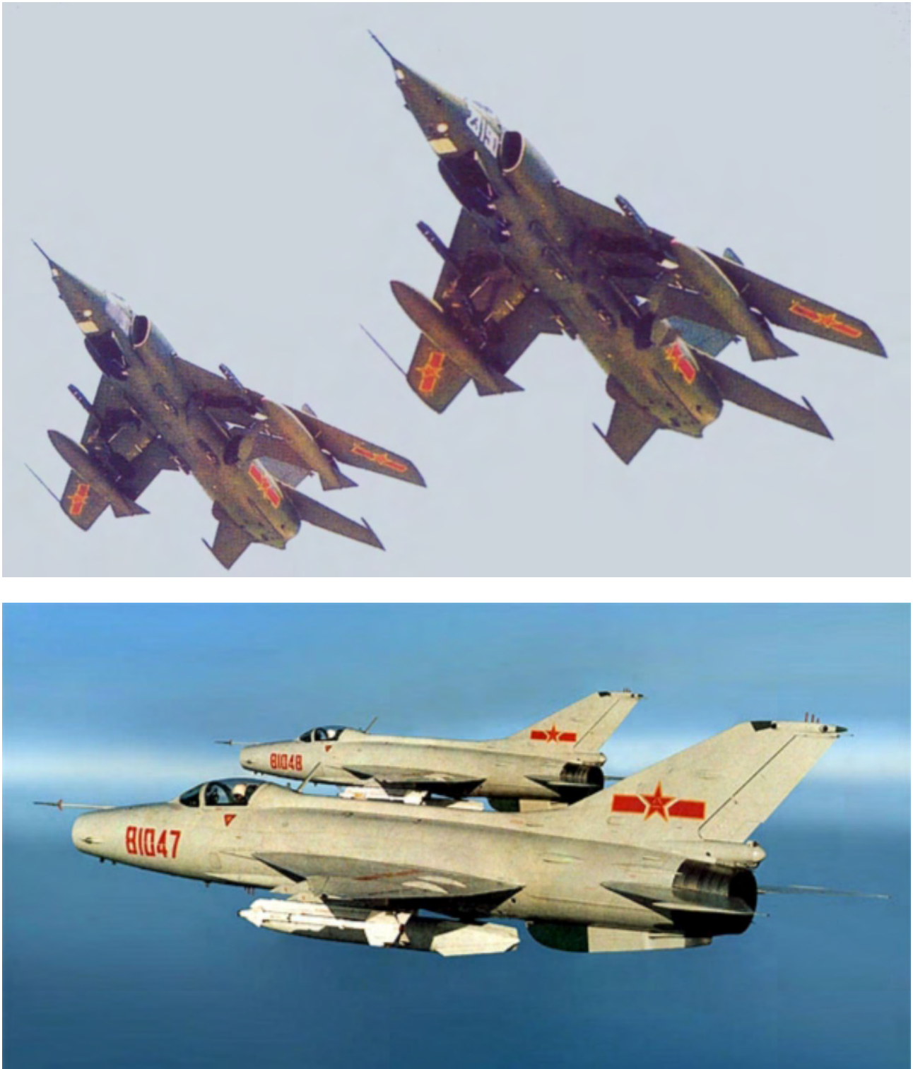
Figure 29: China continues to manufacture and operate a range of legacy types. The Q-5 is an indigenous evolution of the Russian MiG-19 Farmer and is broadly equivalent to the A-4 Skyhawk. Around 600 are in service. The J-7 is an indigenous evolution of the Russian MiG-21 Fishbed and is broadly equivalent to the Northrop F-5 series, but faster and more agile. Around 700 are in service (PLA).
