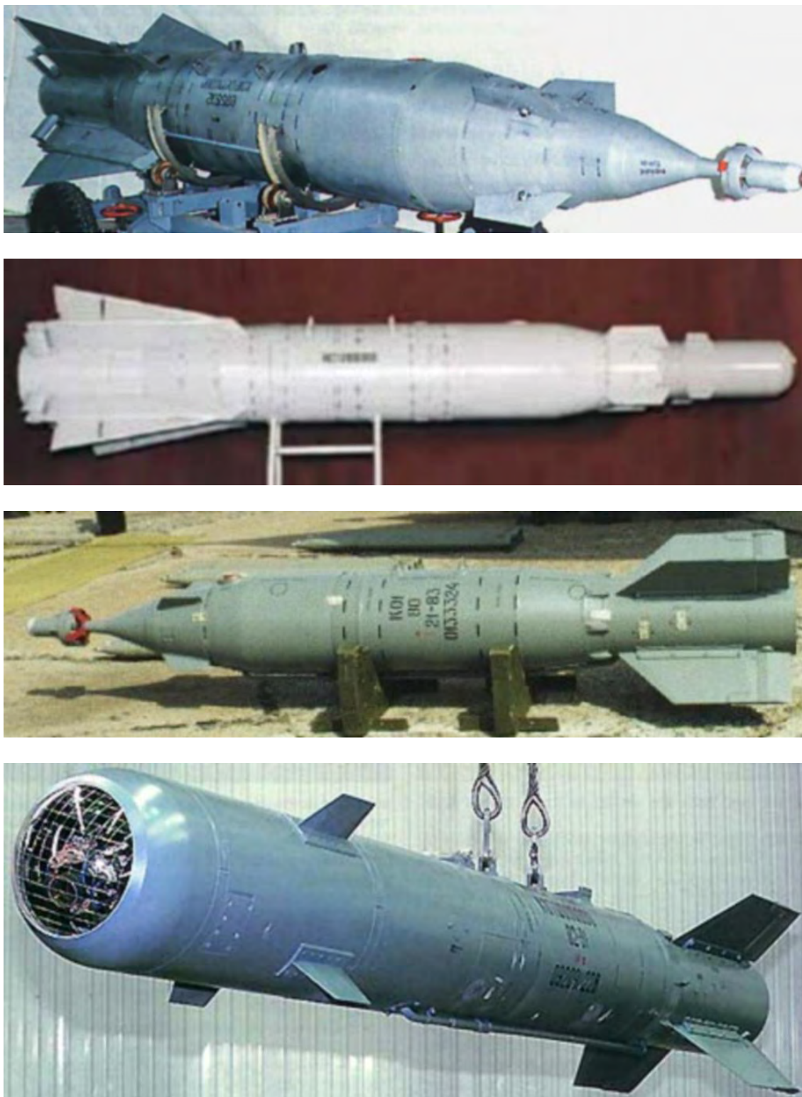
Figure 48: Russia is actively marketing smart bombs for the Sukhoi fleets supplied to the PLA. These images depict the laser and television guided KAB-1500 (1500 kg) series and KAB-500 (500 kg) series guided bombs, available in bunker busting and standard explosive variants. These weapons are broadly equivalent to the US Raytheon GBU-10, GBU-24 carried by RAAF F-111s, and the Boeing GBU-15 which was carried by the F-111 during the 1980s (Rosvooruzheniye).
