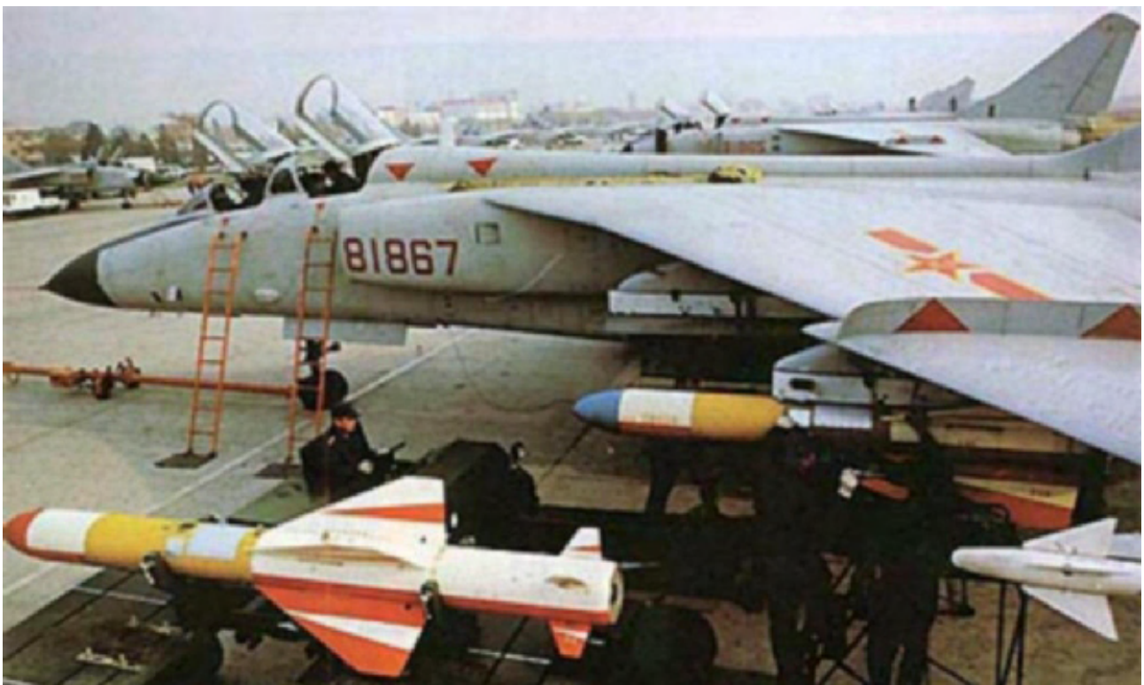
Figure 31: The Xian JH-7 is an indigenous Chinese strike fighter and is broadly equivalent to the RAF Tornado IDS. Around 20 serve with the PLA Naval Air Arm, with the PLA-AF recently taking first deliveries of the enhanced JH-7A variant (PLA).
