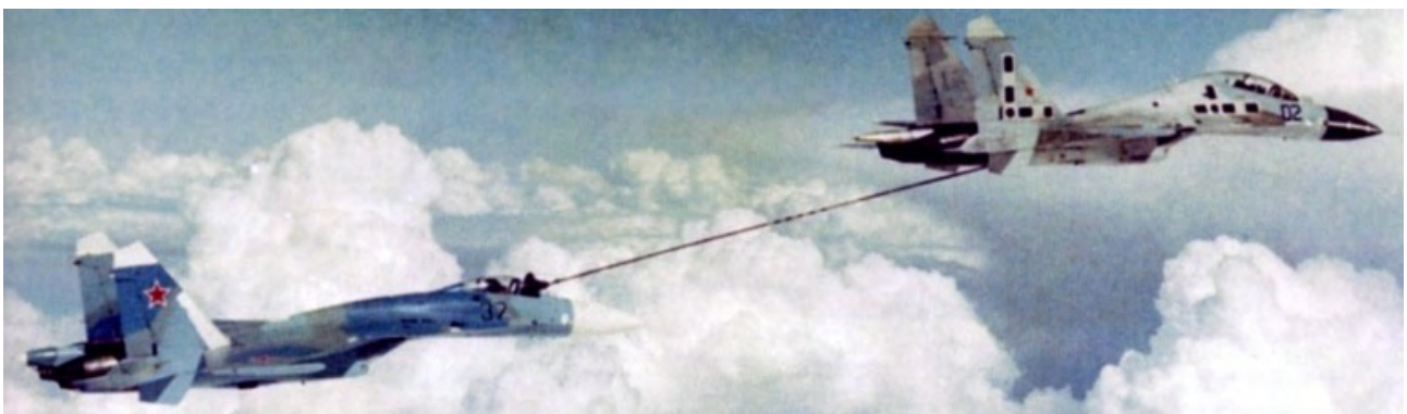
Figure 27: The Il-78MK Midas tanker uses a variant of the UPAZ-1A Sakhalin aerial refuelling pod, which has also been cleared for buddy refuelling on some variants of the Su-27 fighter (RuMOD).
