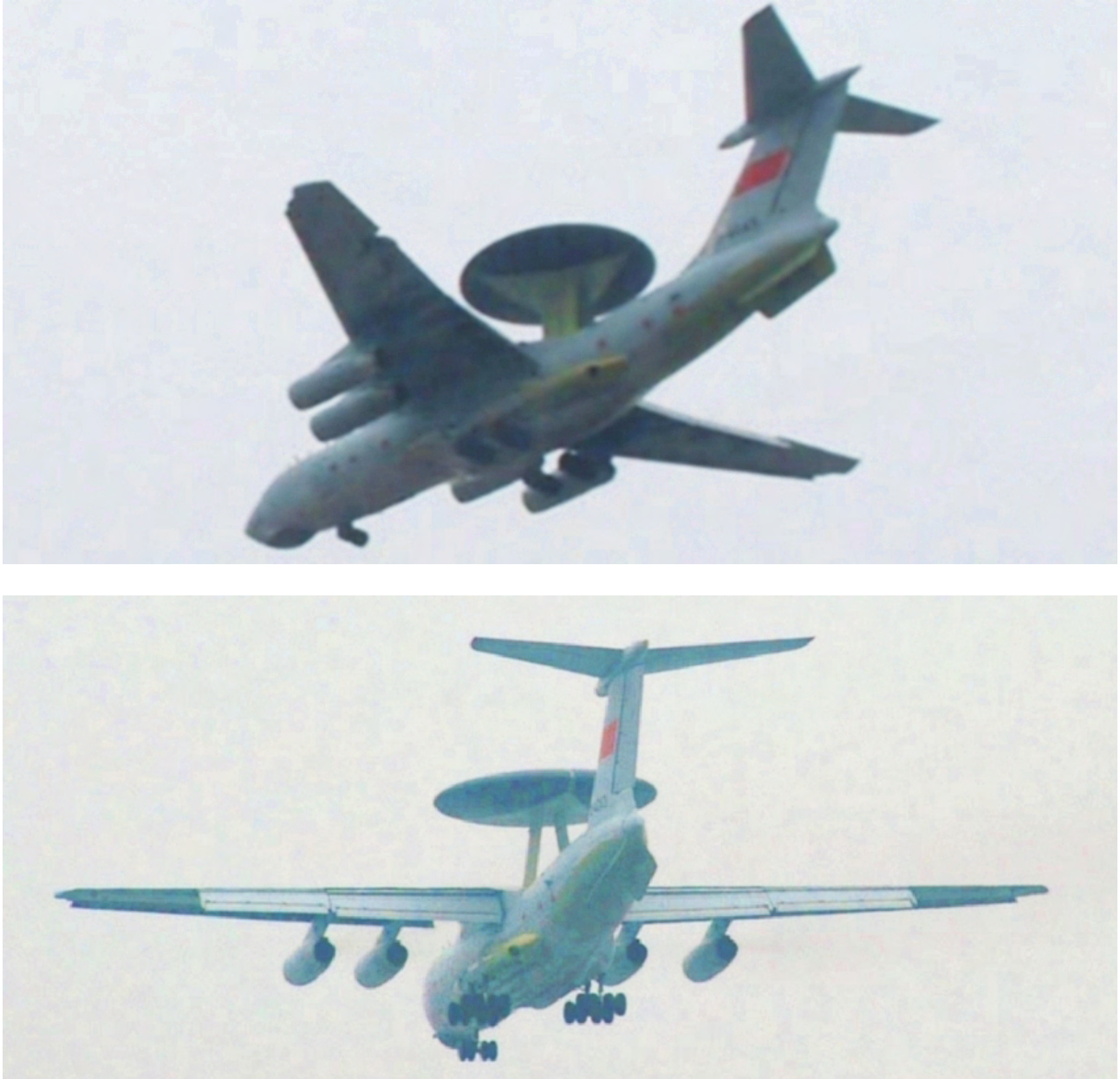
Figure 16: China was reported to have ordered several examples of the Russian A-50E AWACS in the wake of the aborted deal to source the better Israeli A-50I Phalcon variant. Since then photographs have emerged of an indigenous conversion, based in concept on the Israeli A-50I. The images illustrate the use of a phased array radar, similar in technology to the new RAAF Wedgetail - the A-50I radar offered by Israel to China was a variant of the radar offered to Australia for the AIR 5077 bid (via Internet).
