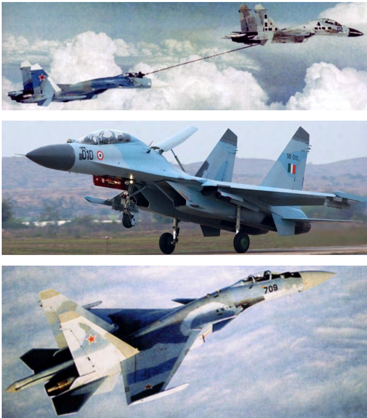
Figure 3: Advanced Flanker variants such as the Su-27SMK Flanker B, Su-33 Flanker D, Su-30MKI/MKK/MKM Flanker G/H and Su-35 Flanker E have key capabilities in common with modern US and EU fighters. These include aerial refuelling probes, buddy refuelling pods, advanced multi-mode radar strike modes, electro-optical targeting systems, digital network modems, glass cockpits and the capability to carry a wide range of smart munitions (Sukhoi, US Air Force).
