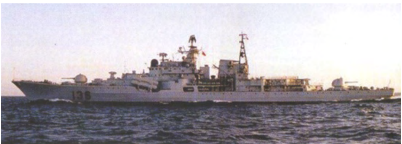
Figure 32: The PLA acquired a pair of 8,000 tonne Type 956E Sovremenniy class destroyers (Hangzhou, Fuzhou), and subsequently ordered another pair. Armed with the supersonic 3M81 Moskit (SS-N-22 Sunburn) cruise missile, these are the most heavily armed warships in the region. In size and capabilities they compare closely to the DDG-51 Arleigh Burke class destroyer (RuMoD).
