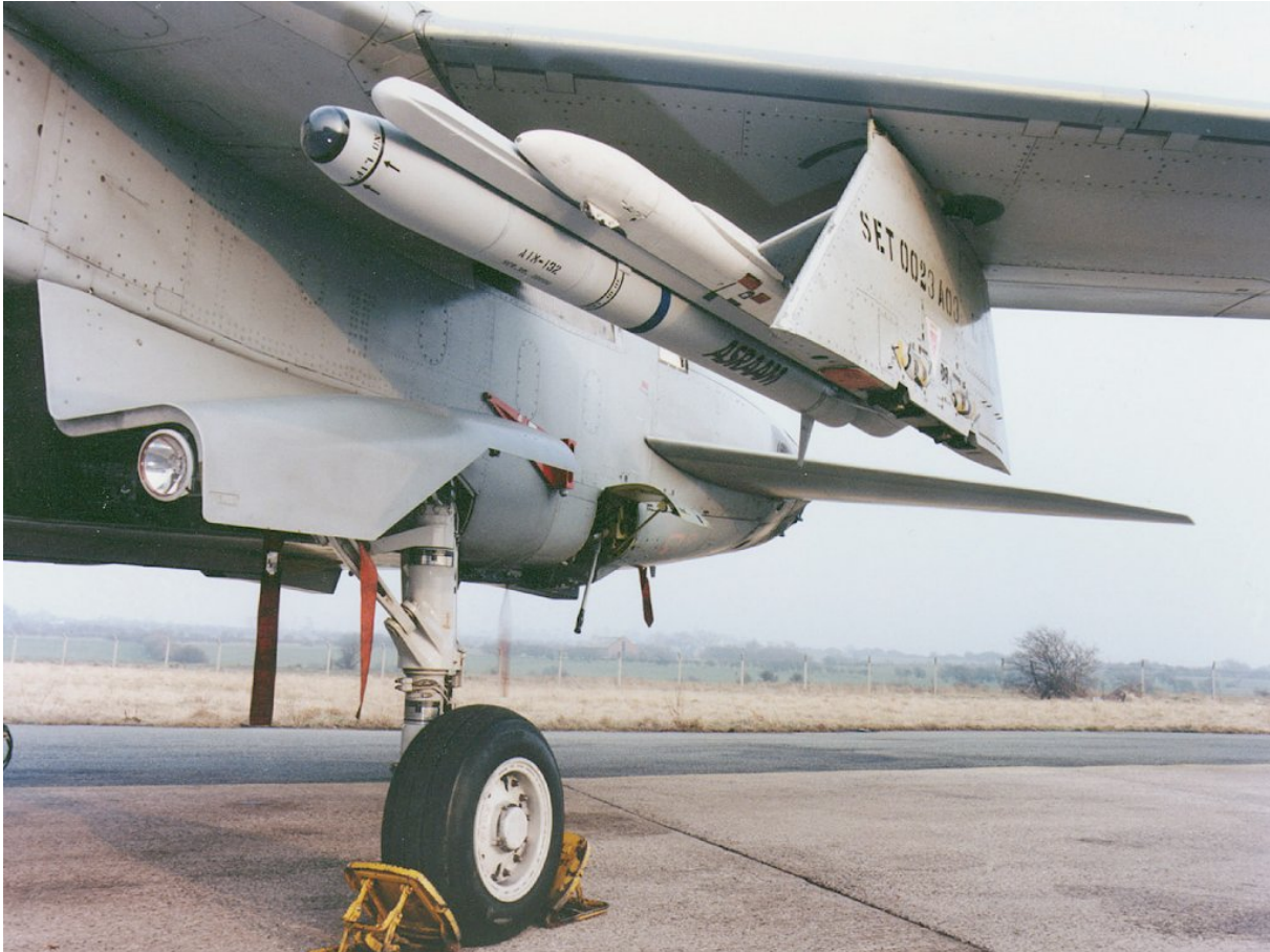
Figure 3: Designed with umbilical interfaces compatible with AIM-9 and AMRAAM, the ASRAAM has similar weight and form factor to the AIM-9. Compared to the AIM-9M, the ASRAAM offers vastly superior range, speed, seeker acquisition performance and agility. Due to its imaging seeker and midcourse guidance package, the ASRAAM has the unique capability to engage a target in the forward and aft hemispheres of the launch aircraft. Engaging a pursuing target requires a helmet mounted sight and swivelling pilot's neck ! (RAF)
