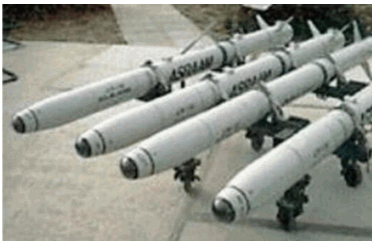
Figure 1: The ASRAAM is arguably a fourth/fifth generation WVR AAM, in that it shares features of WVR and BVR AAMs. The missile employs a midcourse inertial guidance package similar to that in the AMRAAM, but uses a mid-infrared 128 x 128 imaging Focal Plane Array seeker. This allows the missile to be fired at targets beyond visual range, or targets which are not in the Field Of View of the seeker at launch. With a high impulse, short burn motor, the ASRAAM is exceptionally fast and long ranging. (MBDA)
