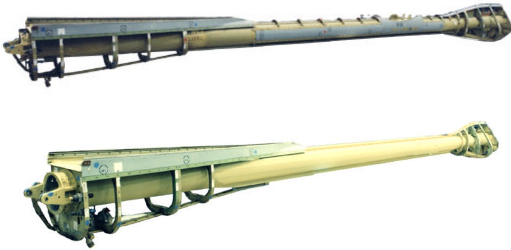
Figure 8. KC-135R Improved Refuelling Boom structural assembly. The “old” KC-135 boom structural tube (upper) has been replaced with a newer single piece extruded component (lower). Externally the appearance of the boom is unchanged (Boeing).
