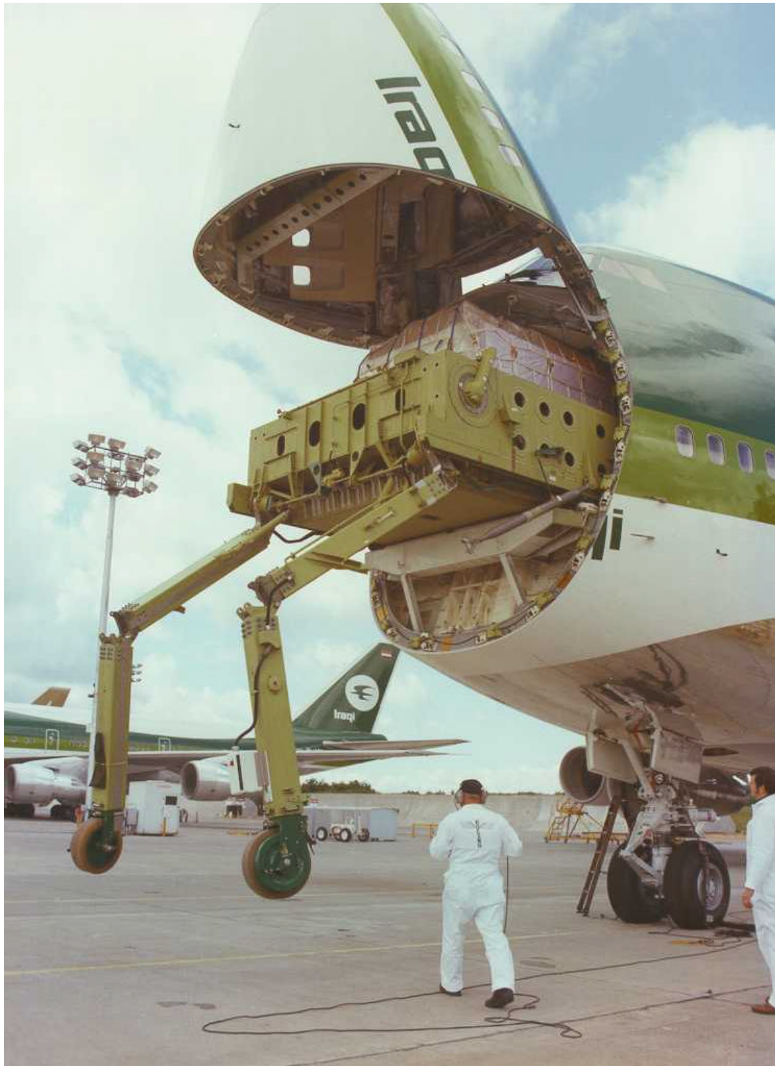
Figure C.8 Boeing On Board Loader, deployment sequence step 3 .
