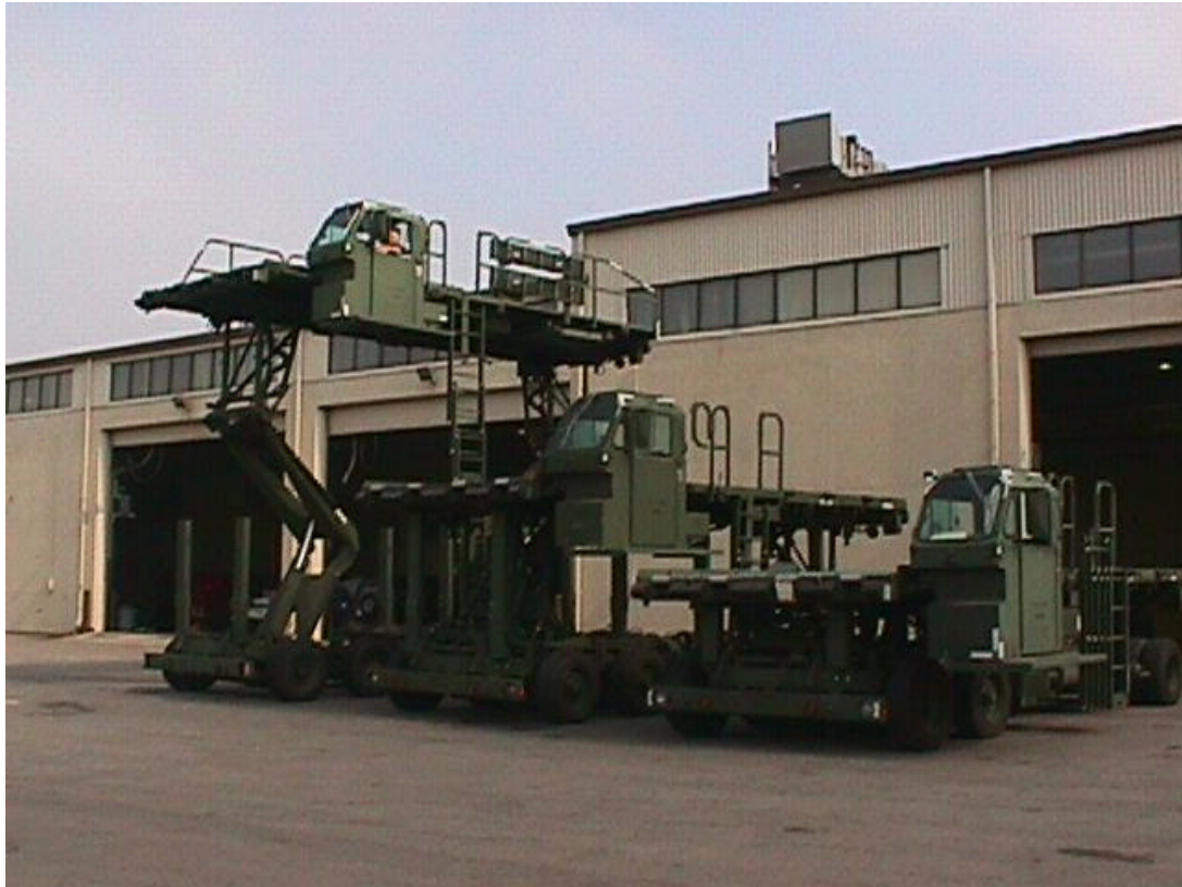
Figure C.19 SEI 25K Loader, up, down and shipping configuration (SEI).
