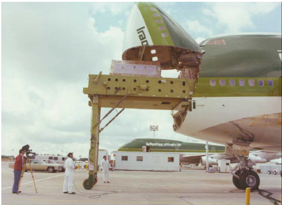
Figure C.10 Boeing On Board Loader, deployment sequence step 5 .
