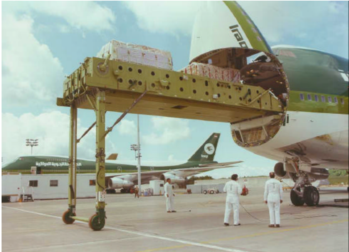
Figure C.11 Boeing On Board Loader, deployment sequence step 6 .
