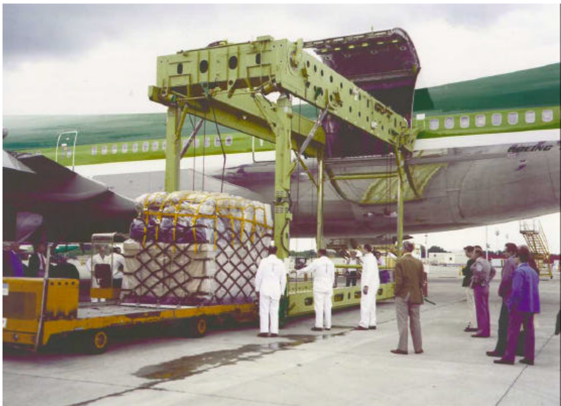
Figure C.4 Boeing On Board Loader, Side Cargo Door pallet loading .
