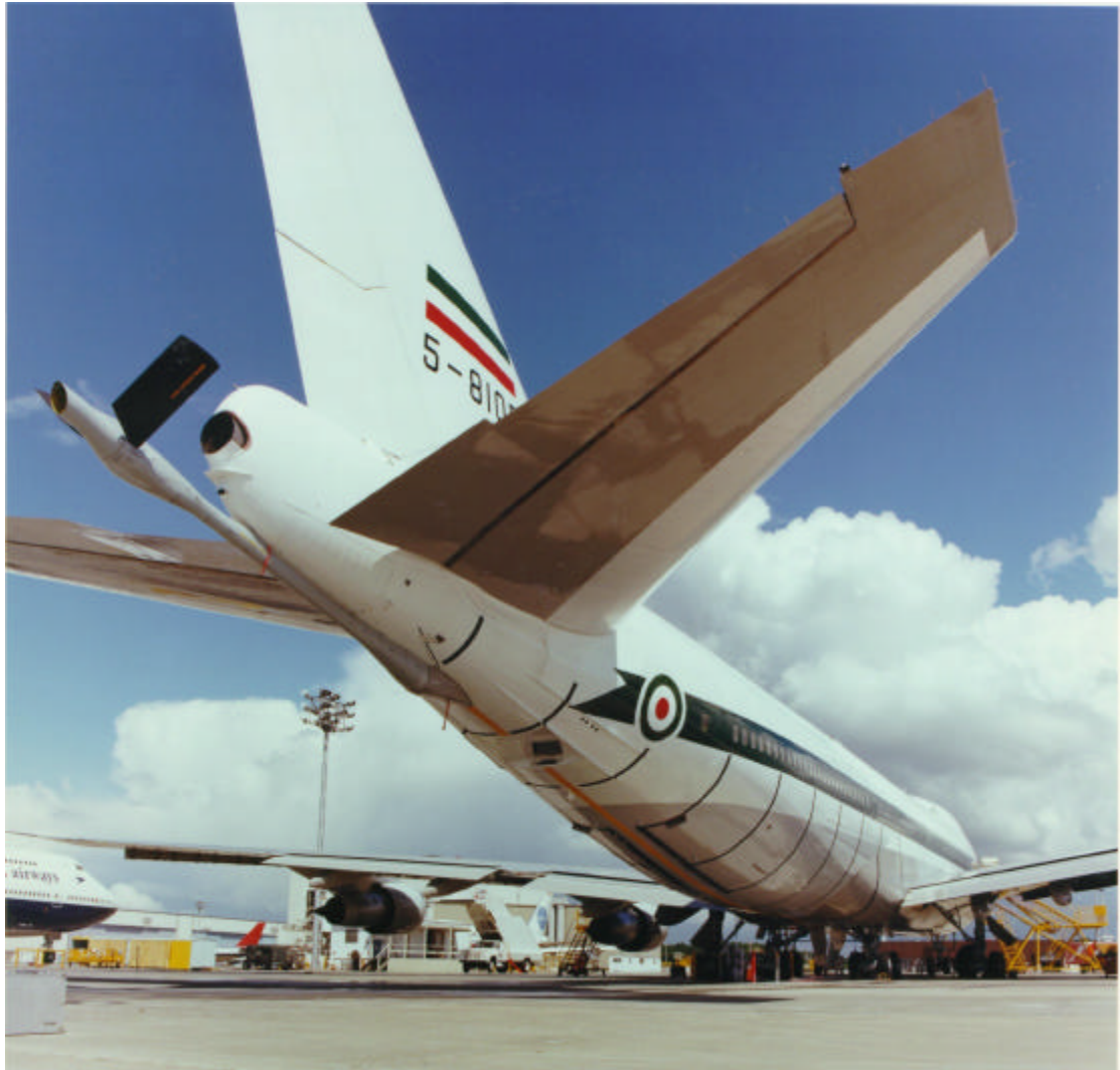
Figure B.7 IIAF KC-747-100 Strategic Tanker/Transport “boomer” station and high speed boom installation (Boeing).
