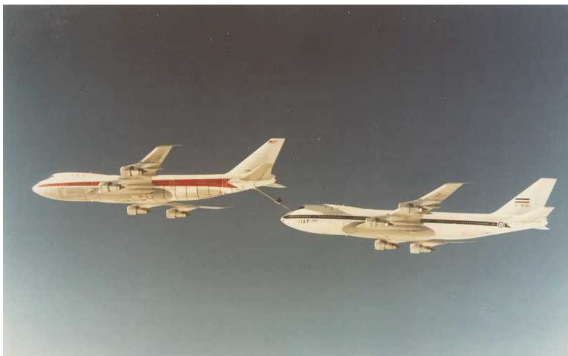
Figure 7. Imperial Iranian Air Force (IIAF) Boeing KC-25/ KC-747-100 Strategic Tanker/Transport refuelling an IIAF 747-100 (Boeing).
