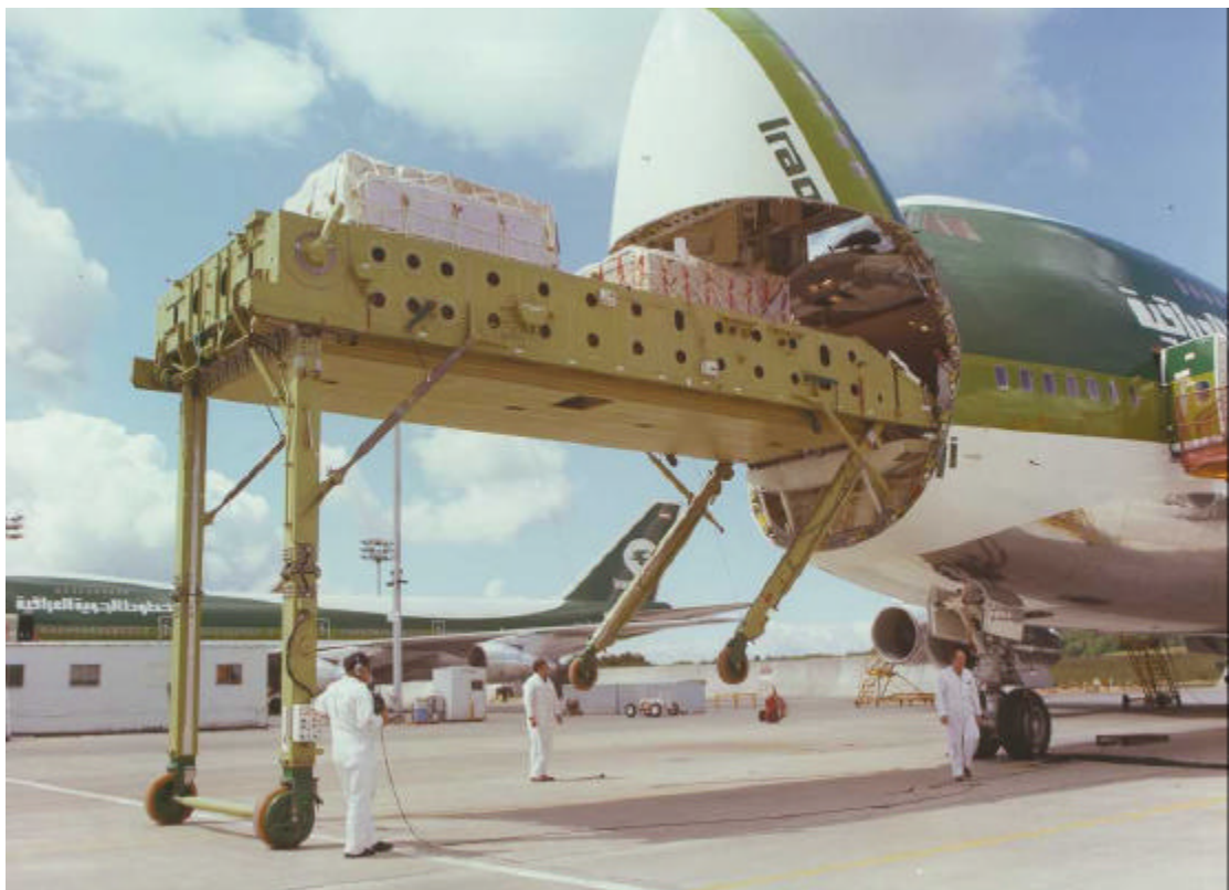
Figure C.12 Boeing On Board Loader, deployment sequence step 7 .
