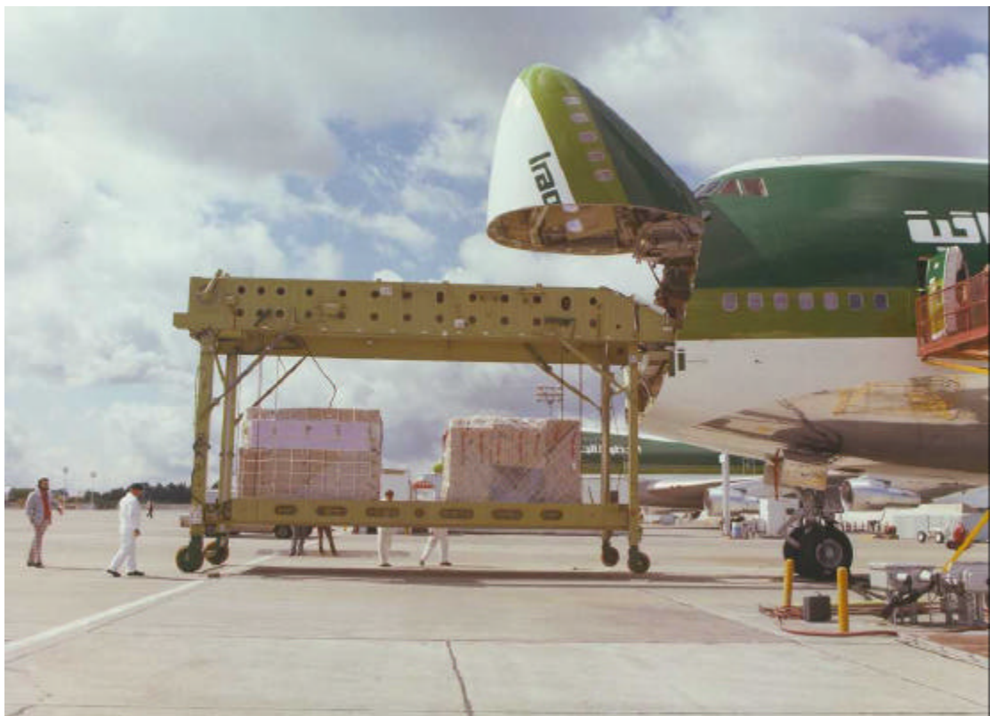
Figure C.2 Boeing On Board Loader, Nose Door loading of palletes .
