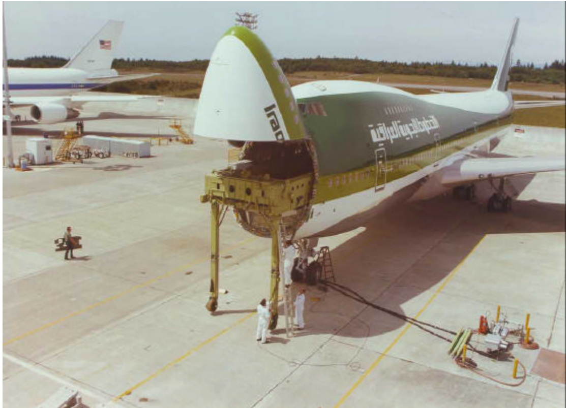
Figure C.9 Boeing On Board Loader, deployment sequence step 4 .
