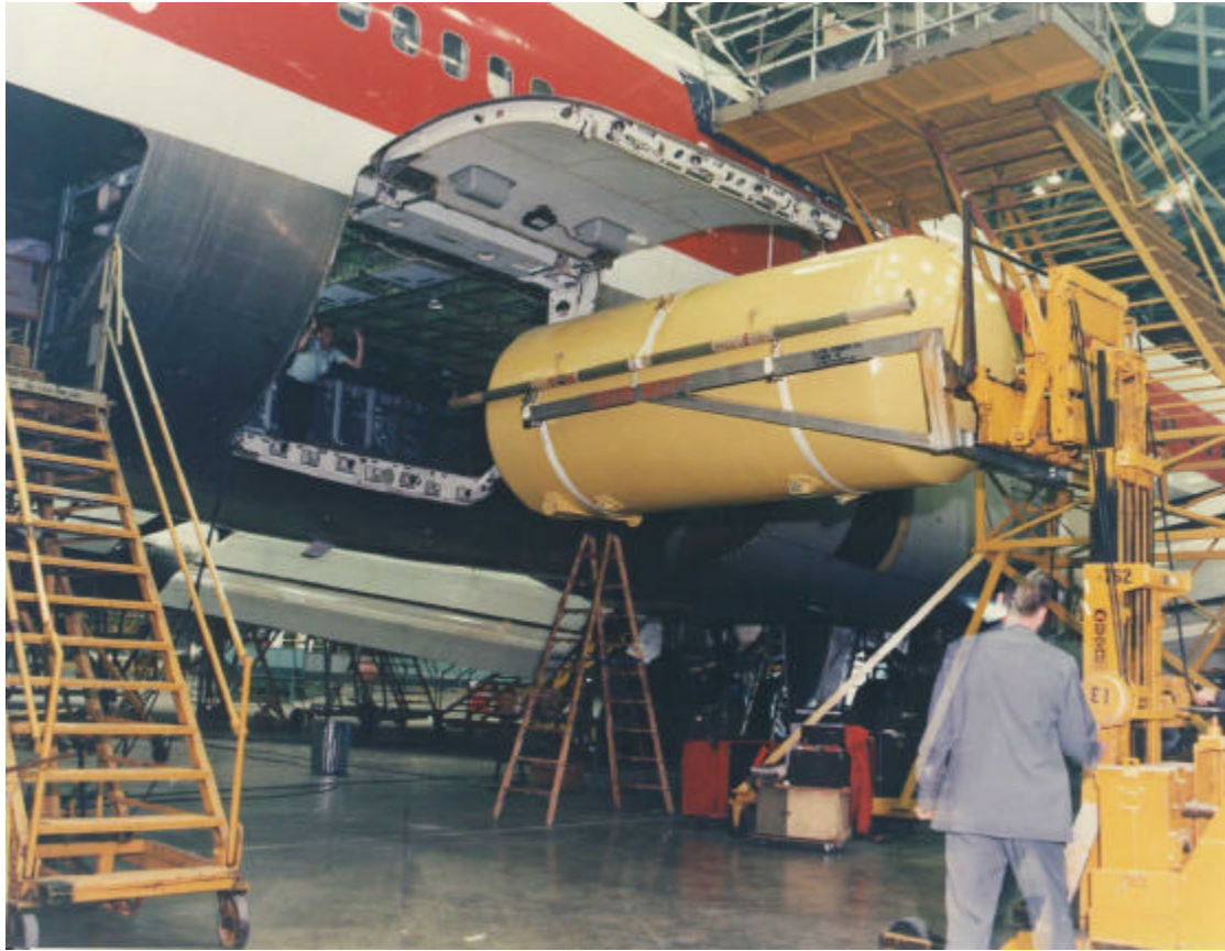
Figure B.5 Installation of a lower deck auxiliary fuel tank in the IIAF Boeing KC-747-100 aircraft. This style of tank design has been superceded by lighter and more maintainable double walled fuel tanks, which have a similar shape and size to the LD2 lower deck luggage container (Boeing).
