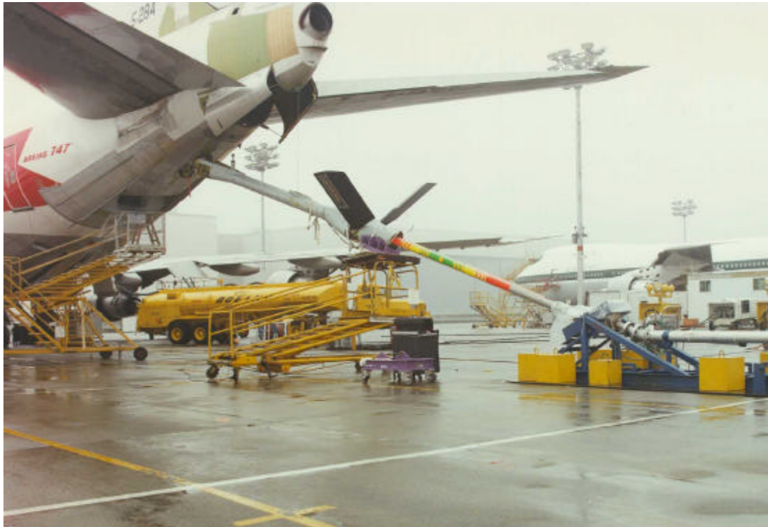
Figure 9. The IIAF KC-25/KC-747-100 boom installation under test. This is an unusually clean installation, with the operator's station recessed in the fuselage. Note the fuselage stiffeners (Boeing).
