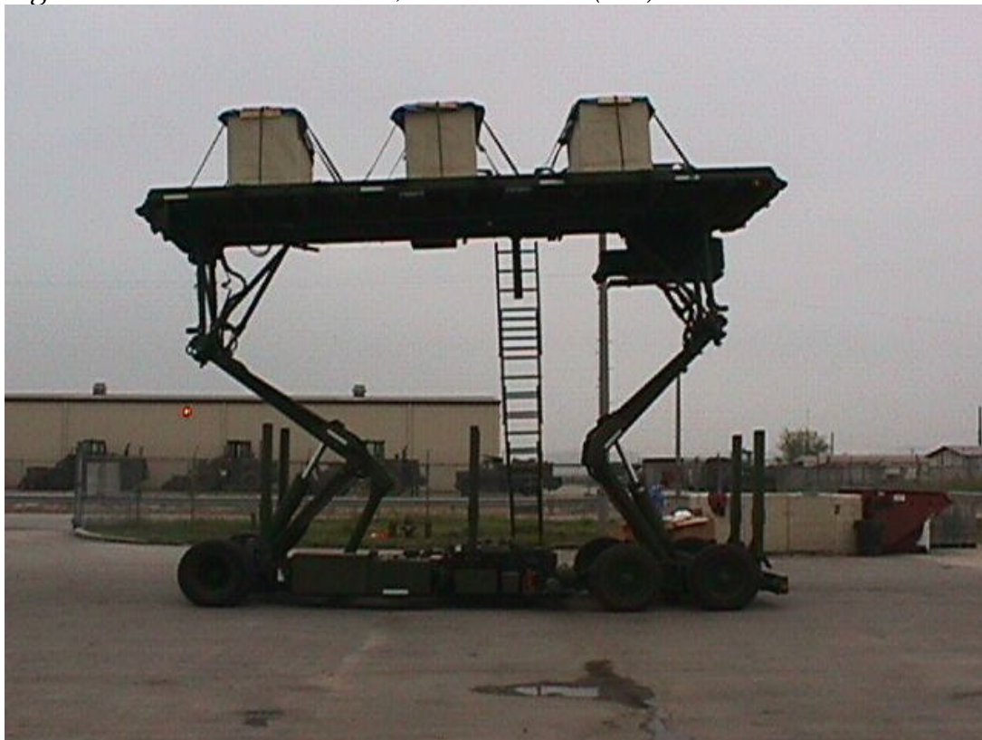
Figure C.17 SEI 25K Loader, front tilt test (SEI).
