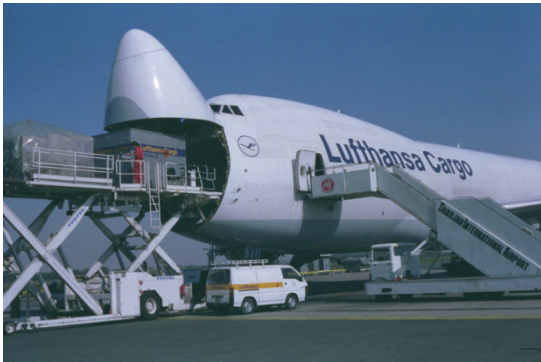
Figure 15. Boeing 747-200F Freighter Nose Door installation being used for container loading. Lufthansa were the lead customer for the 747-100F and remain a major user of the 747-400F (Lufthansa).
