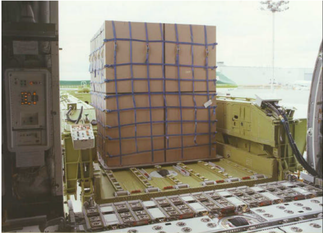
Figure C.5 Boeing On Board Loader, internal view of Side Cargo Door pallet loading operation. Note the generous clearance on either side of the 2.235 metre freight pallet.
