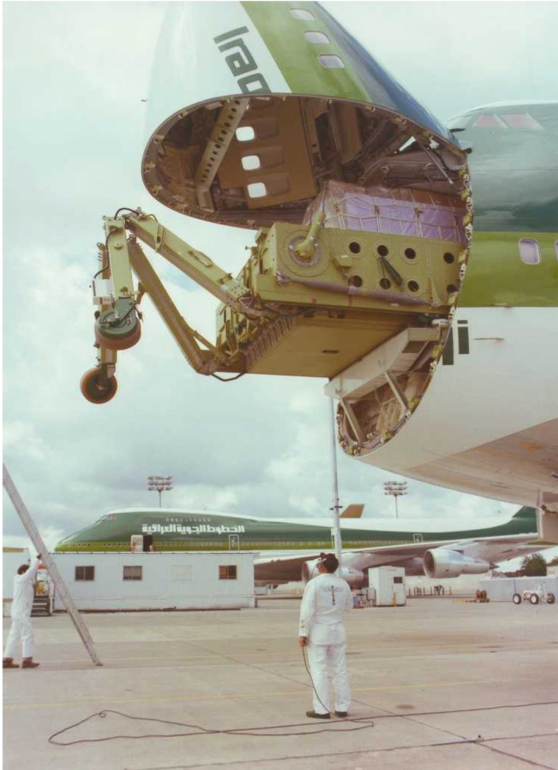
Figure C.7 Boeing On Board Loader, deployment sequence step 2 .
