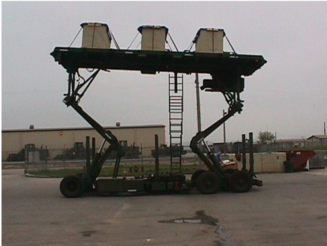
Figure C.17 SEI 25K Loader, front tilt test (SEI).
