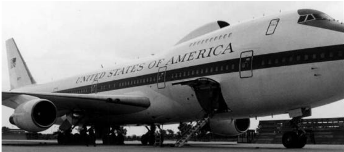
Figure 16. The VC-25A and E-4B both carry internal airstairs to provide crew and passenger access at sites without airliner boarding facilities. The airstairs deploy from the forward cargo door (USAF).
