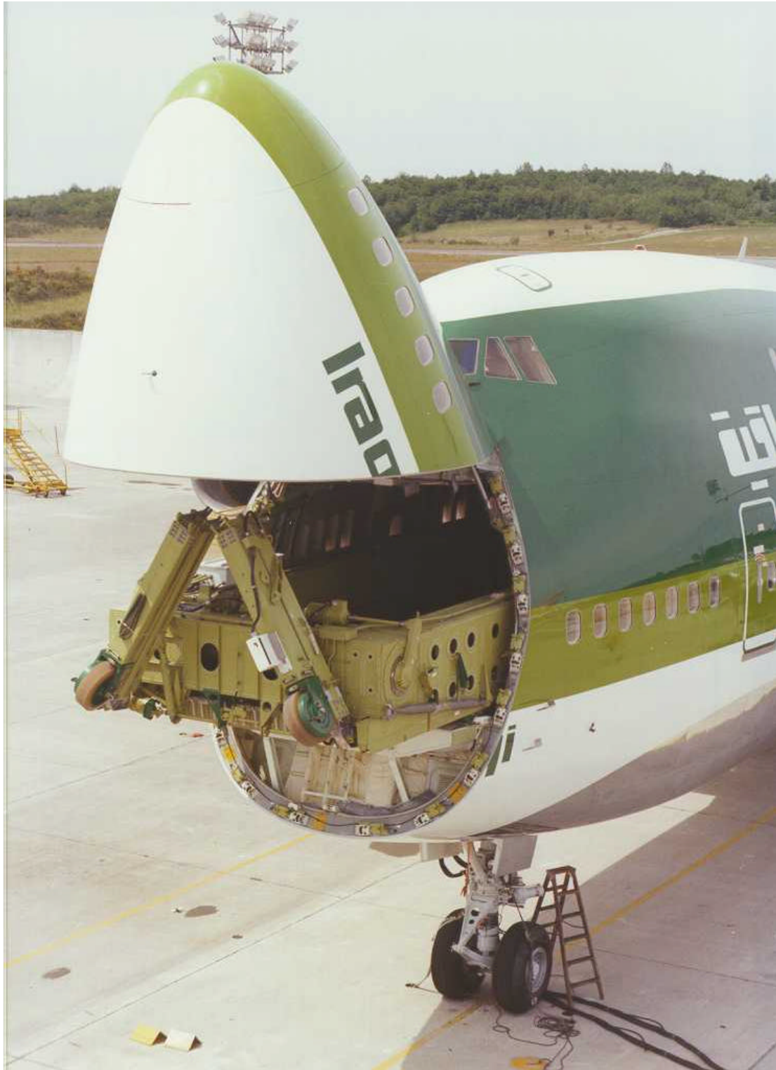
Figure C.6 Boeing On Board Loader, deployment sequence step 1 .
