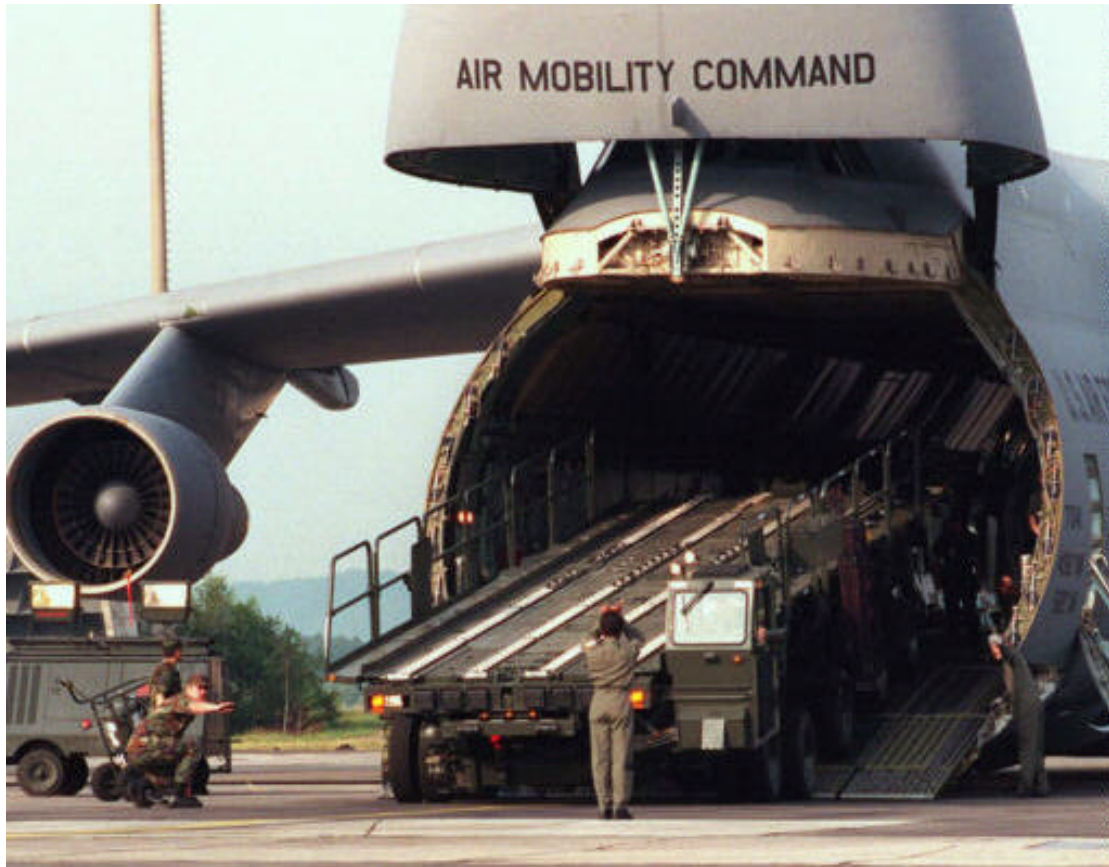
Figure C.15 SEI Tunner Loader, RO/RO deployment in C-5 (USAF).
