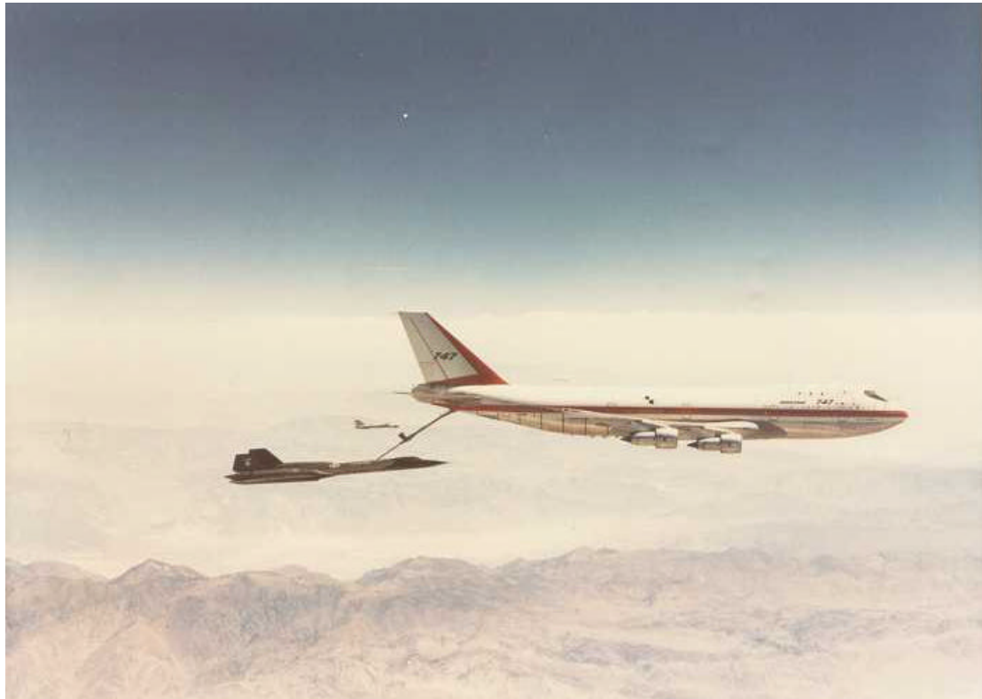
A Boeing KC-747-100 strategic tanker/transport refuelling a USAF SR-71A during inflight refuelling trials. Note the nose down attitude of the tanker. (USAF).
