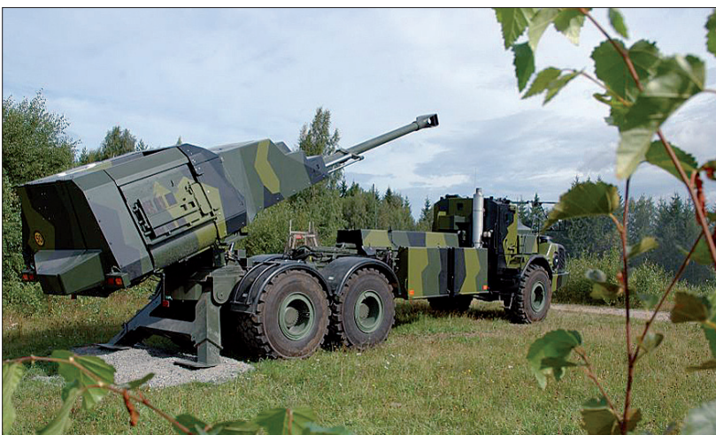
BAE/Bofors FH77 BW L52 Archer self-propelled 155 mm gun – the magazine carries 20 ready to fire rounds.
