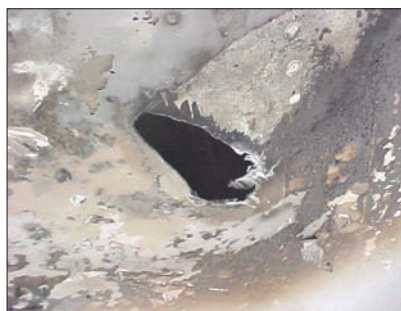
clockwise from above: Target image produced by AIM-9X imaging seeker. Wing tank damage inflicted by shoulder launched missile on DHL Airbus near Baghdad in 2003. R-27ET2 Alamo Heatseeking BVR missile.
