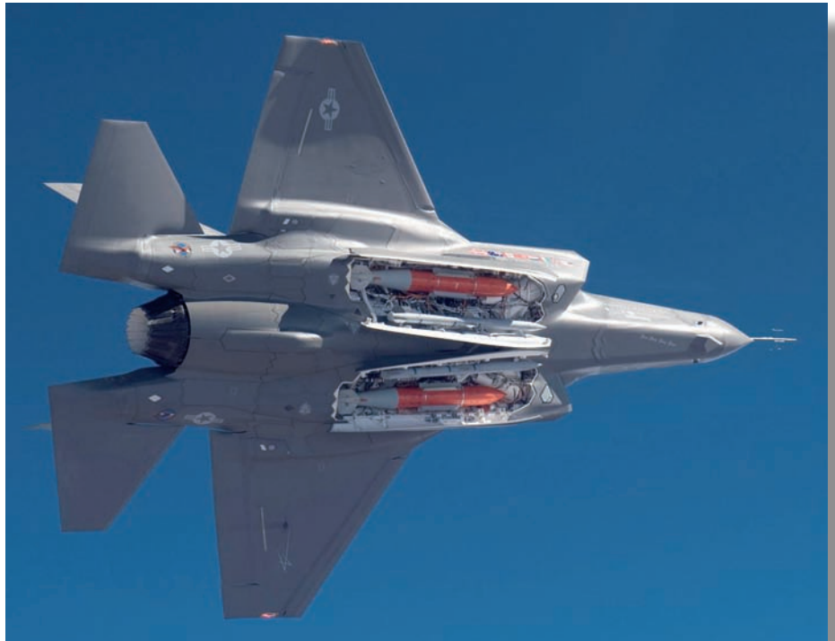
F-35 Joint Strike Fighter with open weapon bays. Note the characteristic hinged bomber style weapon bay doors.
