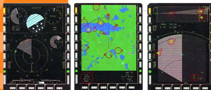
Left: Cockpit multi-function displays in the Gripen fighter cockpit display real-time targeting and situational awareness information to the pilot from which to make decisions about offensive and defensive counter air tactics and weapons employment, or the conduct of attacks against ground targets.
