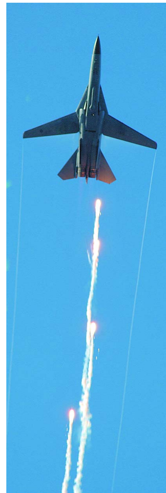
Above: An F-111 releases flares as a countermeasure against surface-to-air missile attack. During the 1980s the RAAF's 82 Wing trialled the 'Precision Air Support' model in which F-111s would orbit at higher altitudes over an area of interest and pick off targets using laser guided bombs, directed by a ground observer. This tactic was embryonic to the 'Persistent Strike' techniques used so successfully in Iraq.
