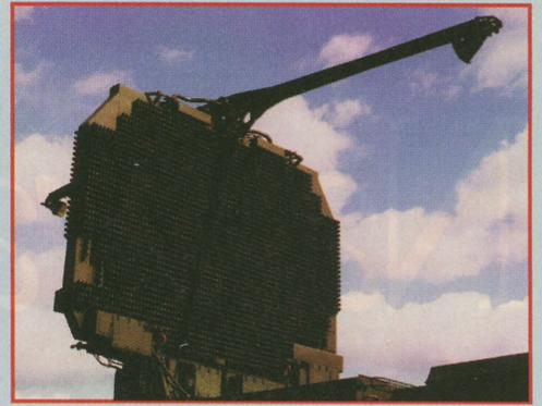
Fig. 2 Big Bird 3D search radar antenna.
