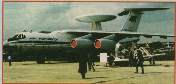
Fig. 28 Mainstay early warning radar aircraft.
