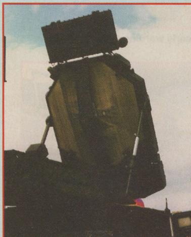
Fig. 17 Rear view of Grill Pan. Metal panel across rear of array is removed for operation.
