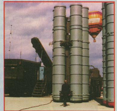
Fig. 9 SA-10 TELAR missile with erected canisters.
