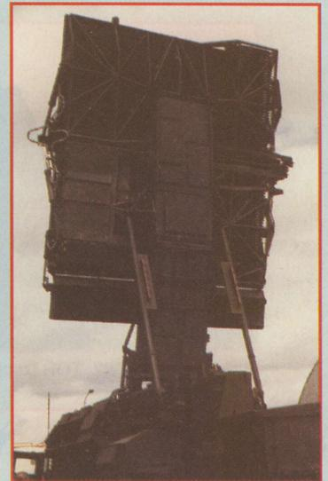
Fig. 15 Rear view of Bill Board array.
