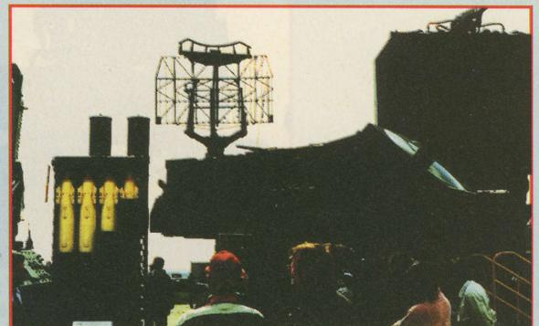
Fig. 20 Side view of TOR vehicle, with missile canister displayed at left, search radar at left end of turret and tracking phased array at right end of turret.
