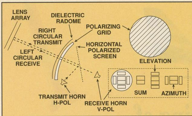
Fig. 8 Sketch of flap lid feed system.
