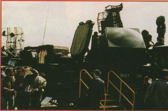
Fig. 22 TOR tracking radar array.
