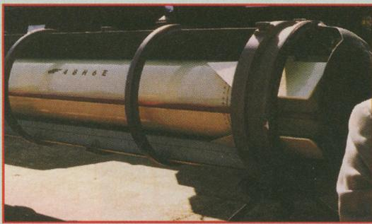
Fig. 10 Tail end of SA-10 missile in canister, showing folded fins and ejection piston rod.
