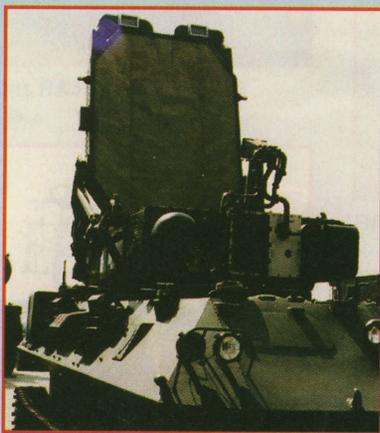
Fig. 24 Zoopark antenna from front, showing complex feed and possible second antenna covered by dome.
