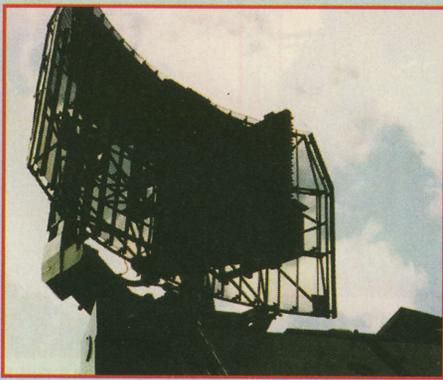
Fig. 21 Front view of TOR search radar antenna.
