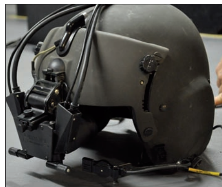
A VSS Virtual Reality display device attached to a pilot's Gentex 56P flight helmet.
