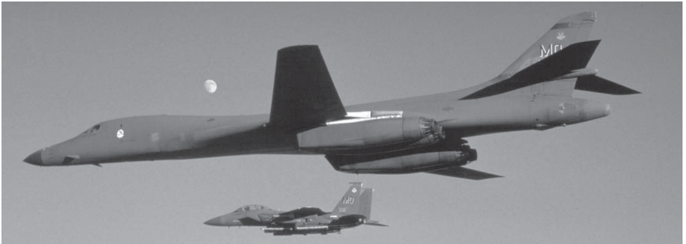
The backbone of the ACC bomber fleet and workhorse of the Afghan battlefield interdiction effort is the Boeing (Rockwell) B-1B Lancer (pictured with an F-15E), of which 100 were built during the Reagan presidency. Evolved around the same penetration model as the older F-111/FB-111, the B-1B carries the largest internal payload of any US bomber. Plagued by ongoing difficulties with its complex electronic warfare package, the B-1B has never been far from controversy. The fleet is currently being downsized with 30 aircraft being mothballed or retired. (US Air Force)
