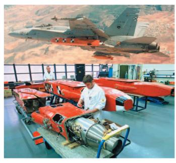
The KEPD-350 is the latest European weapon in the cruise missile class, a development of a family of powered and unpowered standoff weapons. While lacking the stealth of the JASSM, it has been designed from the outset for submunition and unitary warheads, and has a modern guidance package combining GPS, inertial and TERCOM with a thermal imaging terminal seeker. (EADS)
