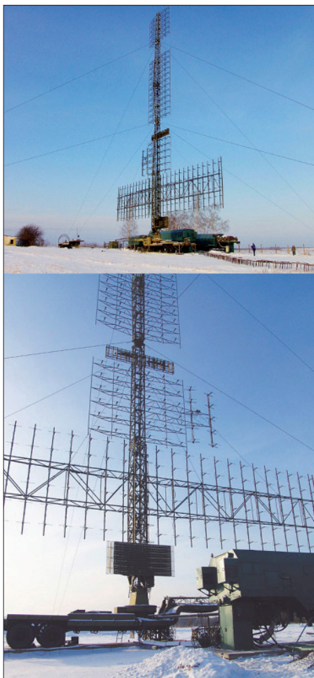
The massive 55Zh6 Nebo UE Tall Rack is the largest VHF 3D radar in production, and is being deployed around Moscow to support S-400/SA-21 missile batteries. While difficult to deploy, it has high angular resolution and range performance (NNIIRT image).
