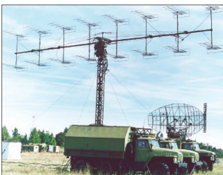
The UHF band P-15 Flat Face was a mainstay of the Cold War period. A digital variant, the Kasta 2E1, remains in production, and digital upgrades are available for legacy models.
