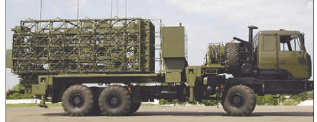
The KB Radar (Agat) Vostok E is an entirely new 2D VHF radar design, using a unique wideband "Kharchenko" square ring radiating element design, in a diamond lattice pattern. With fully hydraulic leveling and deployment, the radar can be operating 8 minutes after coming to a stop. It is the most mobile VHF design ever built, rivaling L/S/X-band 'shoot and scoot' missile battery radars.
