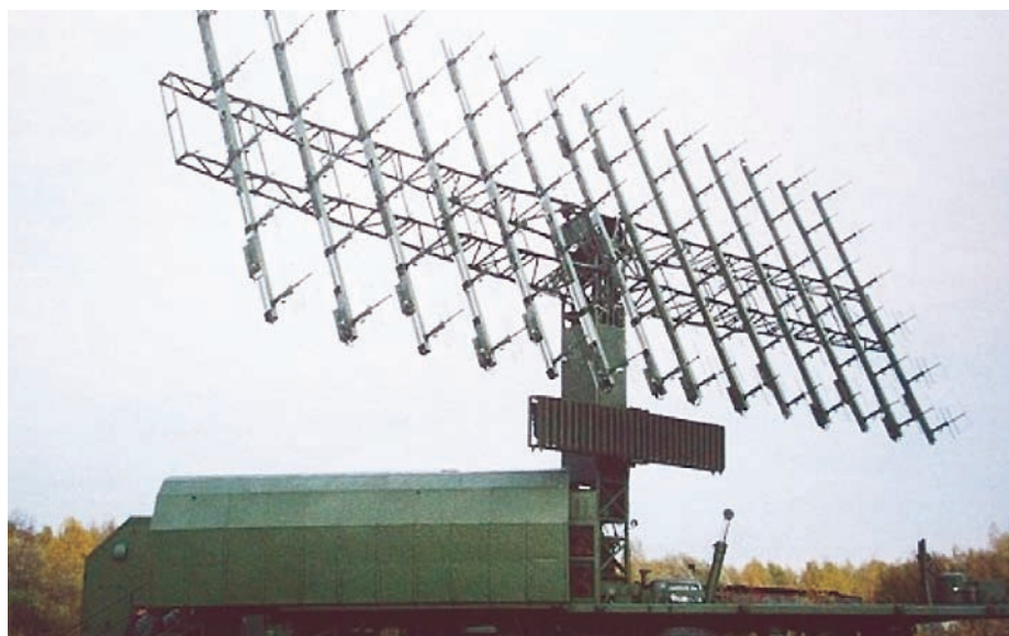
Russian VHF radars. It is a fully digital AESA with precision 3D capability, with accuracy rivaling S-band missile battery acquisition radars.
