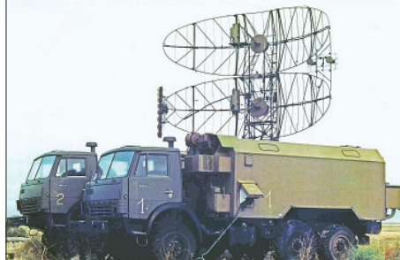
The UHF band P-15 Flat Face was a mainstay of the Cold War period. A digital variant, the Kasta 2E1, remains in production, and digital upgrades are available for legacy models.
