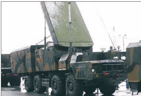
Late model self propelled 30N6E Flap Lid B radar.
