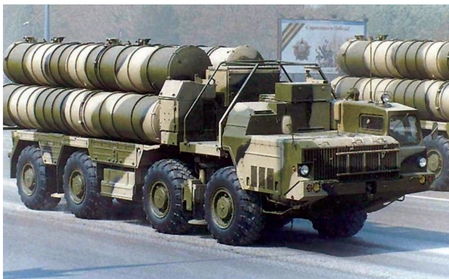
High mobility 5P85SE Transporter Erector Launcher from an SA-10C SAM battery.
