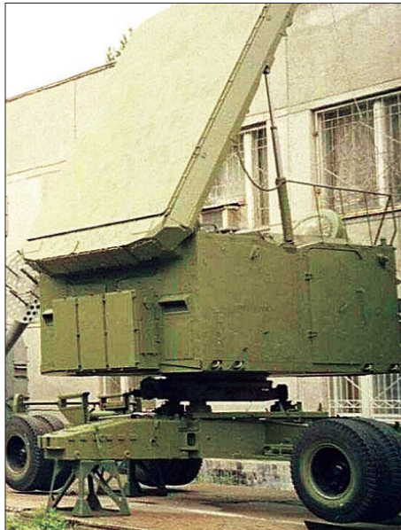
Early model towed 5N63 Flap Lid A radar.
