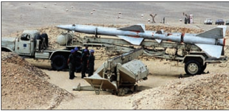
SA-2 PR-11A transloader and SM-63 launcher.
