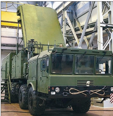
Late model 92N6 Grave Stone engagement radar.
