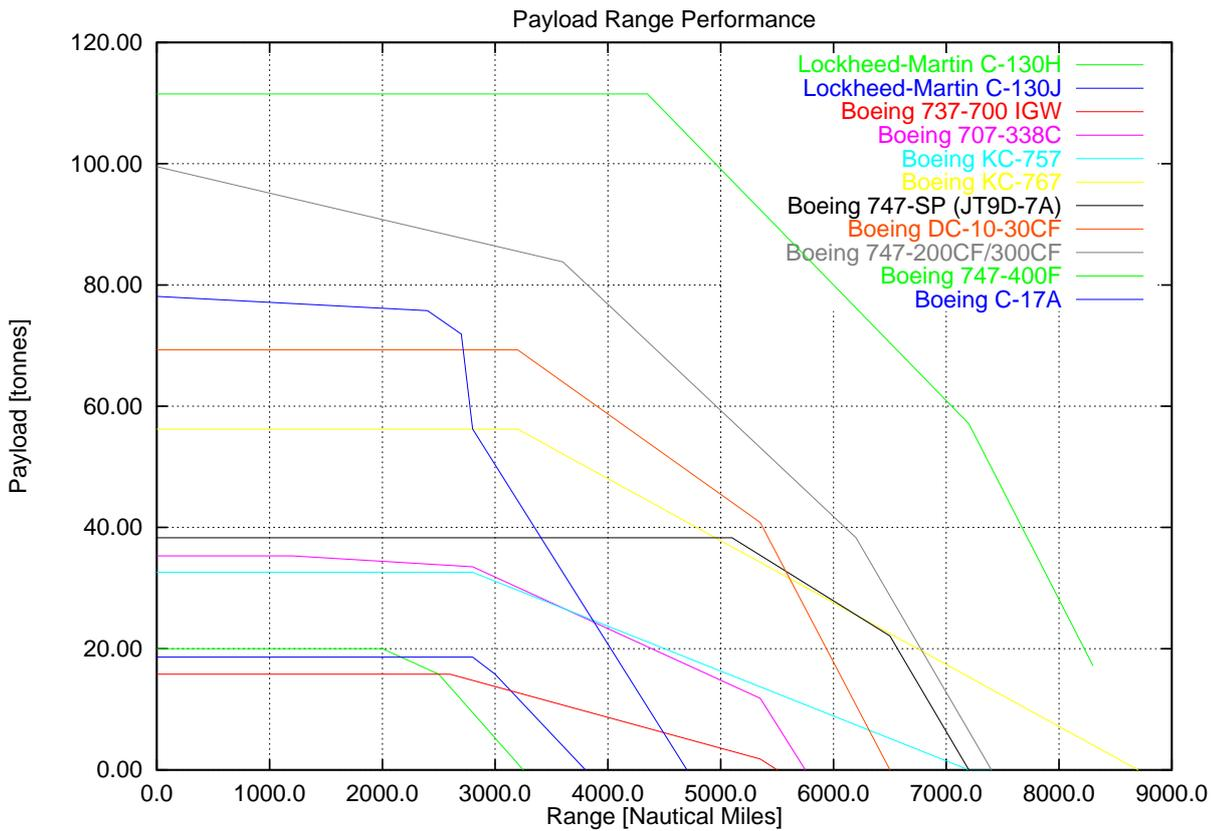
Figure 16: Comparison of payload/radius performance for representative aerial refuelling aircraft (Author, Boeing and other data).
