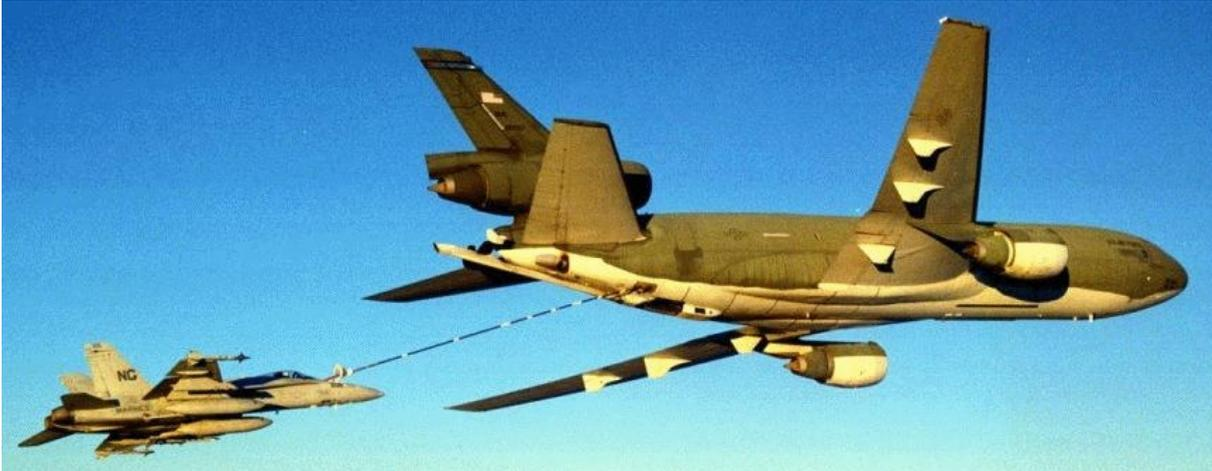
Figure 10: *The Boeing (MDC) KC-10A is based on the DC-10-30CF airframe, which was superseded by the MD-11. With the recent completion of MD-11 production, the supportability of the US Air Force's 59 strong KC-10A fleet will be compromised once most of the commercial DC-10-30 fleet is retired in the 2010-2015 period, if not earlier due to the airline industry collapse (US Air Force).*
