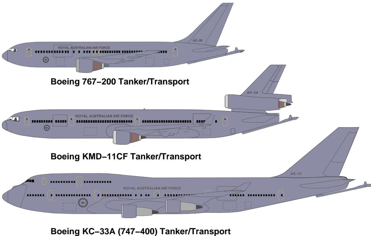
Figure 15: *Size comparison of the Boeing 767-200, KMD-11 and 747-400 series tanker/transports (Author).*
