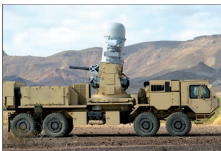
Phalanx C-RAM system. While highly effective in the C-RAM role, this system lacks necessary improvements to perform effectively in the C-PGM role.
