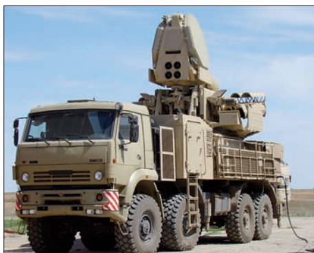
The latest variant of the Russian KBP 96K6 Pantsir S1 SPAAG incorporates a Janus-faced phased array acquisition radar specifically developed to defeat saturation attacks by high speed guided munitions.
