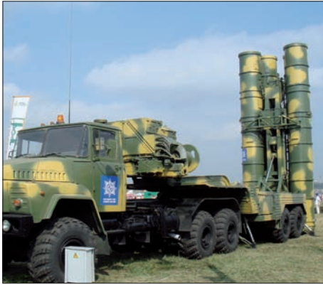
5P85TE TEL used with SA-20A and some SA-20B systems.
