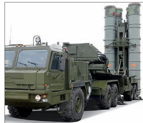
5P85TE2 common TEL used with the SA-20B and SA-21 SAMs.
