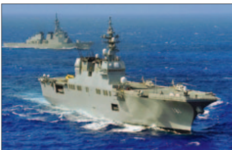
The Japanese Hyuga class DDH is a 19,000 tonne class ASW helicopter carrier. Two larger 27,000 tonne DDH vessels are under construction, intended to embark up to 14 SH-60K Seahawk ASW helicopters. While Japan is planning to use its DDH classes to perform both ASW and amphibious roles, there are no known plans for analogous dual role amphibious and ASW utilisation of the Canberra class LHDs.
