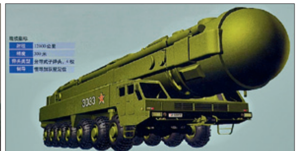
Two distinct TEL designs have been credited to the DF-41 MIRV ICBM. The fourteen wheel design is entirely new, but the sixteen wheel design appears to be based on the WS2400 family of TELs.
