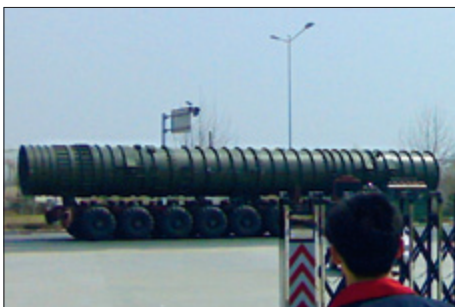
Two distinct TEL designs have been credited to the DF-41 MIRV ICBM. The fourteen wheel design is entirely new, but the sixteen wheel design appears to be based on the WS2400 family of TELs.
