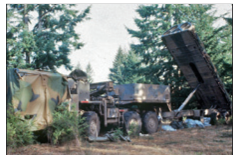
GLCMs like this scrapped 1980s US Air Force BGM-109G Gryphon are extremely difficult to kill once dispersed to hides. The CJ-10 provides a unique capability in this respect, as the United States and Russia are forbidden by treaty to deploy such weapons.
