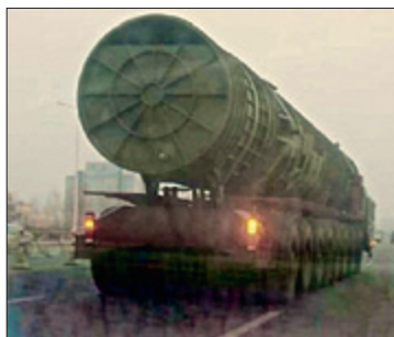
Two distinct TEL designs have been credited to the DF-41 MIRV ICBM. The fourteen wheel design is entirely new, but the sixteen wheel design appears to be based on the WS2400 family of TELs.
