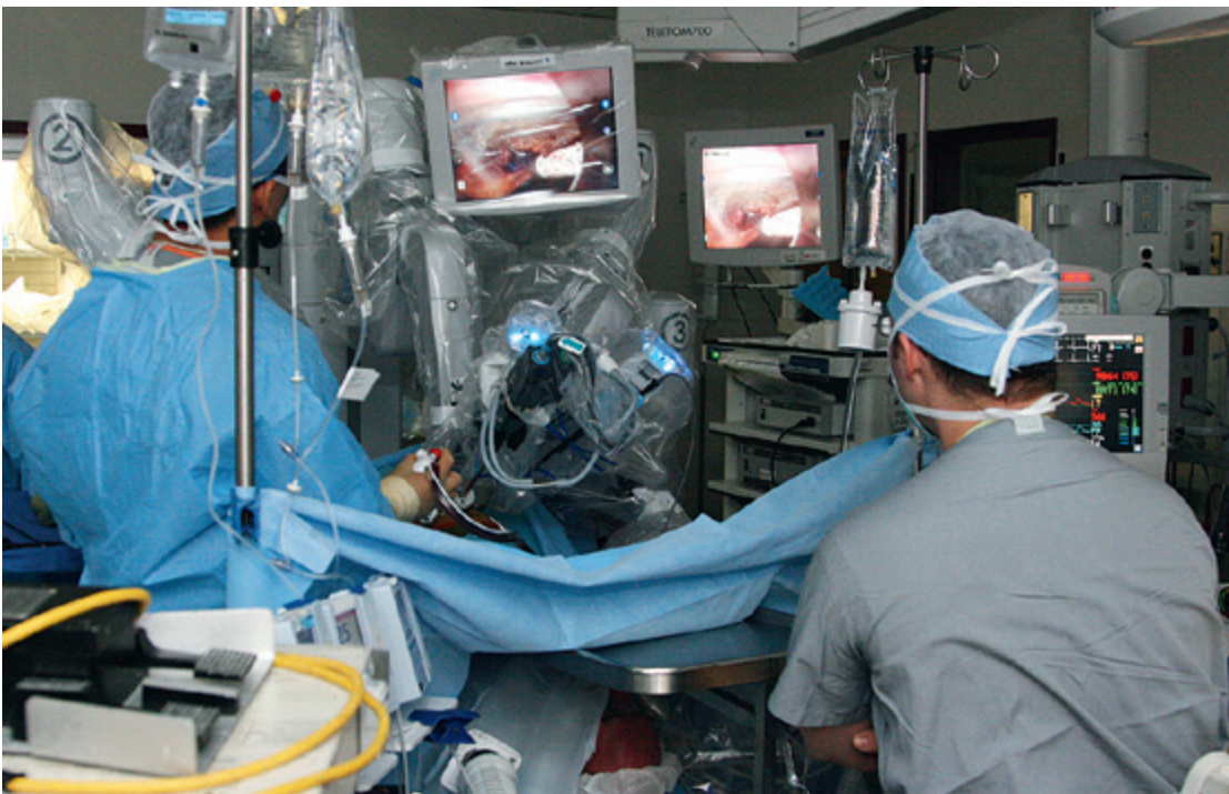
Surgeons at United States Walter Reed Army Medical Center in Washington, D.C., using a robotic surgical station. Remote control of surgical robots permits specialist surgeons to treat injuries in theatre which would otherwise require the patient be flown out of theatre.
