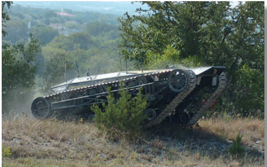
The RIPSAN-MS1, designed to be an unmanned convoy security vehicle, demonstrates its off-road capabilities during a lanes exercise at the US Army Fort Hood Robotics Rodeo, September, 2009. The RIPSAN is equipped with six claymore mines, can carry 2.3 tonnes of payload and tow multiple military vehicles.
