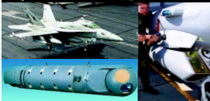
AIR 5376 OPTIONS: From top left - Raytheon ATFLIR pod on US Navy ‘Hornet’; Lockheed Martin ‘Pantera/Sniper XR’-derivative pod and Northrop Grumman’s ‘Litening’ advanced targeting pod (bottom left)
