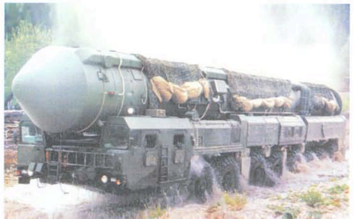
Russian road-mobile SS-27 is carried in a canister on a new eight-axle transporter-erector-launcher.
