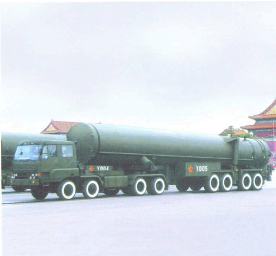
China is continuing development of the new DF-31 road-mobile ICBM (a three-stage, solid-propellant missile carried inside a canister).
