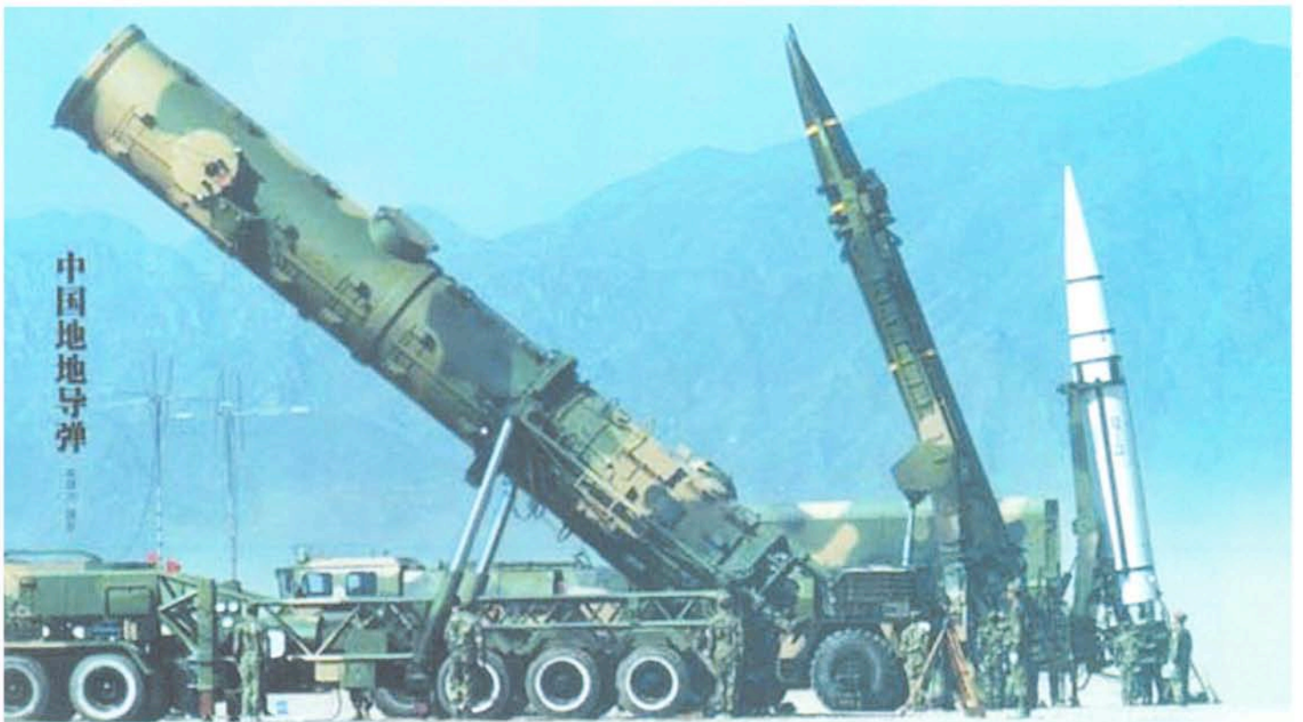
Chinese Road-Mobile Missiles (left to right) CSS-5 MRBM (missile is inside canister), CSS-7 SRBM, and CSS-6 SRBM
