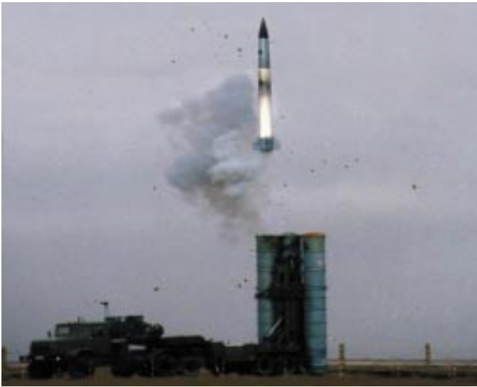
The S-300P series systems use a 'cold launch' technique where the missile is ejected from the launch tube and its motor initiated once it is clear. This dramatic shot shows a late model 48N6E missile launching from a 5P85TE series road mobile TEL. Note the raised datalink antenna behind the KrAZ-260B tractor cab. (Rosvooruzheniye)
