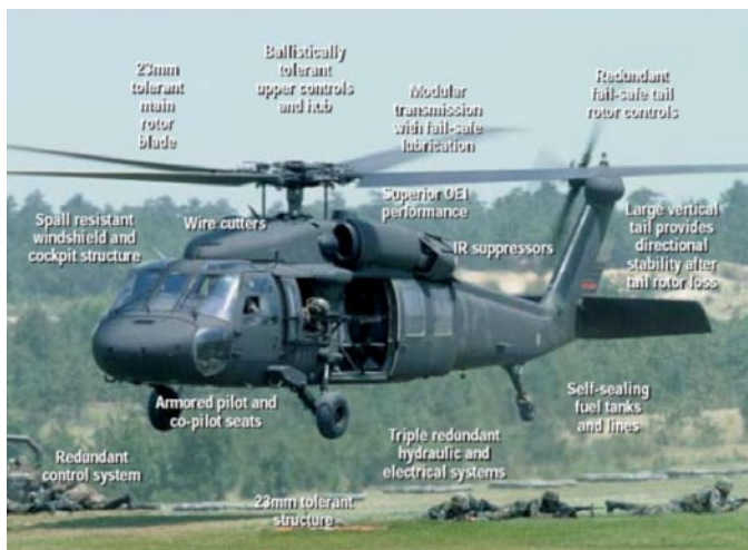
Following appalling losses of UH-1 and AH-1 helicopters during the Vietnam conflict, the US Army defined tough survivability requirements for the UH-60 Black Hawk and AH-64 Apache. The ballistic tolerance and crashworthiness requirements for the UH-60 have become the defacto benchmark followed by most modern military helicopter designs. (Sikorsky)
