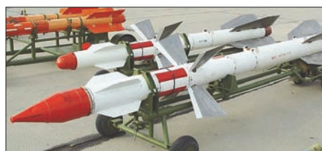
A short burn heatseeking R-27T and long burn semi-active homing R-27ER1.
