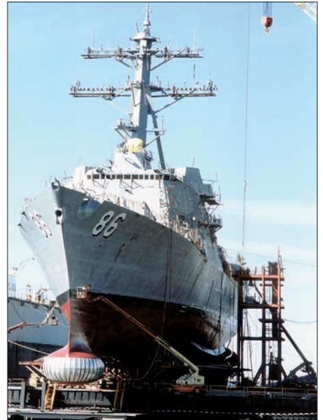
Late build Arleigh Burke class destroyer bow active sonar array.
