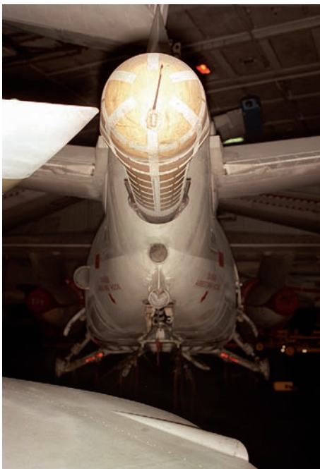
A rear view of the ASQ-81 Magnetic Anomaly Detection (MAD) boom on an S-3A Viking.
