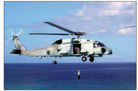
Raytheon AN/AQS-22 ALFS carried by an MH-60R Seahawk.
