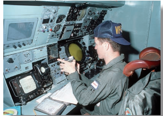
Magnetic anomaly detection (MAD) equipment in the P-3 Orion.
