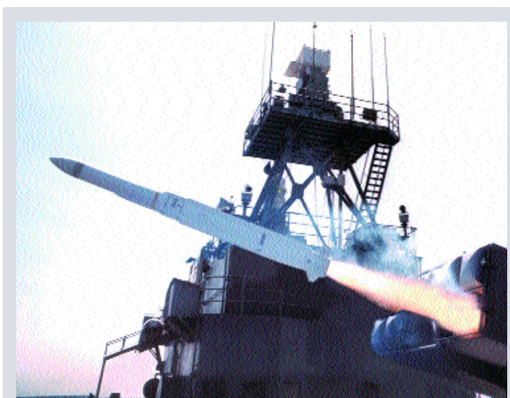
The RIM-162 Evolved Sea Sparrow Missile is the weapon of choice for engaging sea skimming Anti-Ship Cruise Missiles. Developed in an international program, the missile employs terminal X-band semi-active homing guidance with midcourse datalink updates. A single Mk.41 VLS cell can be loaded with an insert carrying four ESSM rounds, to maximise weapon loadout (Raytheon).
