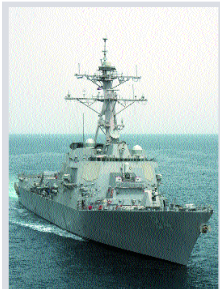
The DDG-51 Arleigh Burke class destroyer is regarded by many to be the leading contender for SEA 4000. Equipped with the SPY-1D AEGIS system, late build examples displace over 9,000 tonnes full load. The US Navy plans to operate 48 examples, replacing the DDG-2 class (US Navy).
