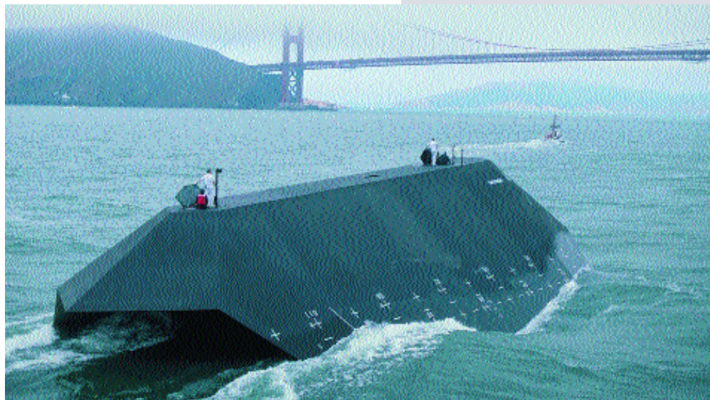
Lockheed's 1980s Sea Shadow technology demonstrator was the first ever 'stealth warship'. Anecdotes from the period claim it was so stealthy, it could be detected as a 'black hole' in the ocean wave clutter background (Lockheed-Martin).
