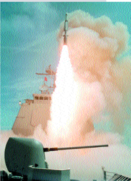
The Block IV RIM-66 Standard Missile is being developed as an anti-ballistic missile interceptor, intended to engage Tactical and Intermediate Range Ballistic Missiles. Note the additional booster stage and enlarged strakes (Raytheon).
