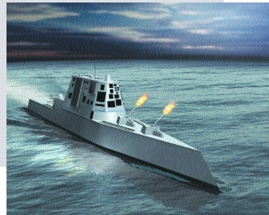
The US Navy's new 12,000 tonne class Northrop-Grumman DD(X) destroyers will be the first of a new generation of surface combatants incorporating a wide range of technological innovations. Two of these are of particular interest. The first is the integrated 'dual band radar' suite combining the active phased array X-band SPY-3 MFR and S-band Volume Search Radars, both sharing a common back end for antenna control and processing. The SPY-3, also planned for the CG(X) and a wide range of larger vessels, is designed to defeat saturation missile attacks. The wave piercing hull shape and superstructure is designed for stealth from the outset, resulting in a much lower radar signature than any current warships (US Navy/Northrop-Grumman).
