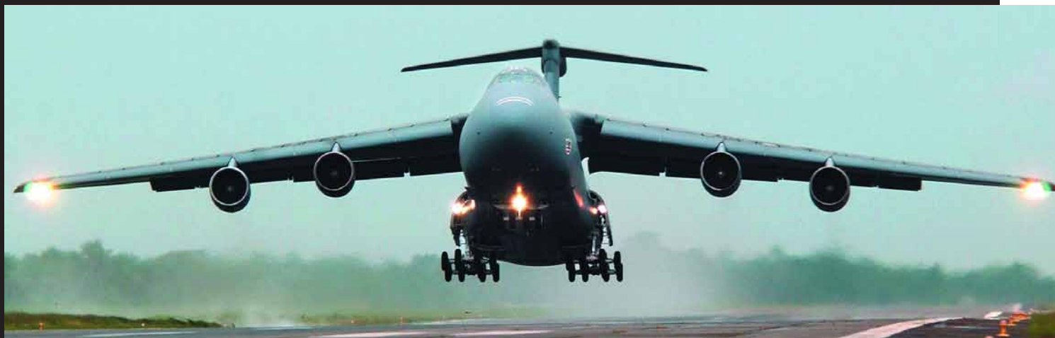
The C-5 is the largest RORO airlifter in US service, set to remain in operation until the 2040 period. The most recent upgrade is likely to see CF-6 engines, widely used on the 747, replacing the legacy powerplants.
