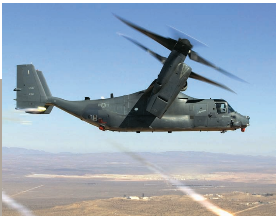
After long, troubled and expensive development the MV-22 Osprey is entering US service. It provides amazing performance, combining flight characteristics of helicopters and conventional winged aircraft but at a cost and with unanswered safety concerns.
