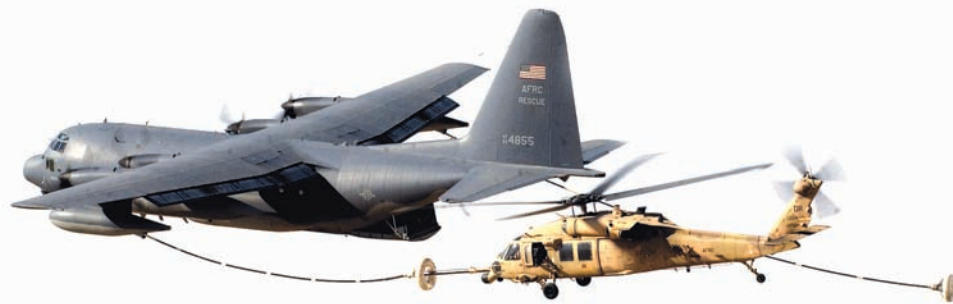
Using in-flight refuelling of helicopters is an alternative way of filling the battlefield airlift capability rather than acquiring a new aircraft type. (USAF Photo)
