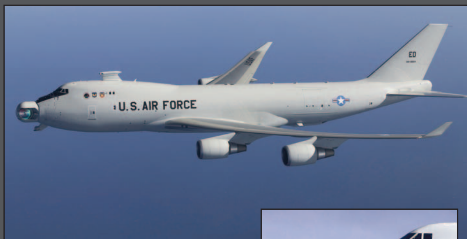
The YAL-1A ABL prototype carried in a Boeing 747-400F airframe of the United States Air Force.
