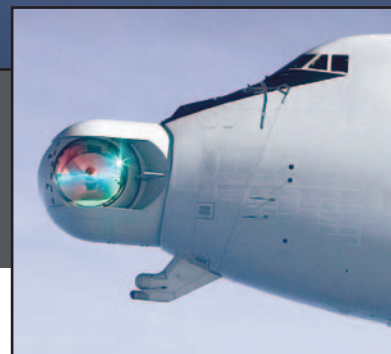
The YAL-1A ABL prototype carried in a Boeing 747-400F airframe of the United States Air Force.
