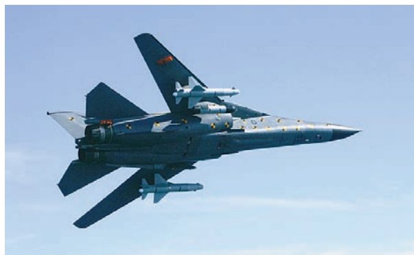
The most important recent development in the F-111 world was the successful test firing of the AGM-142E Stand Off Weapon, using the new Block C-4 Mil-Std-1760 based digital weapon system, designed to support the latest digital weapons.
