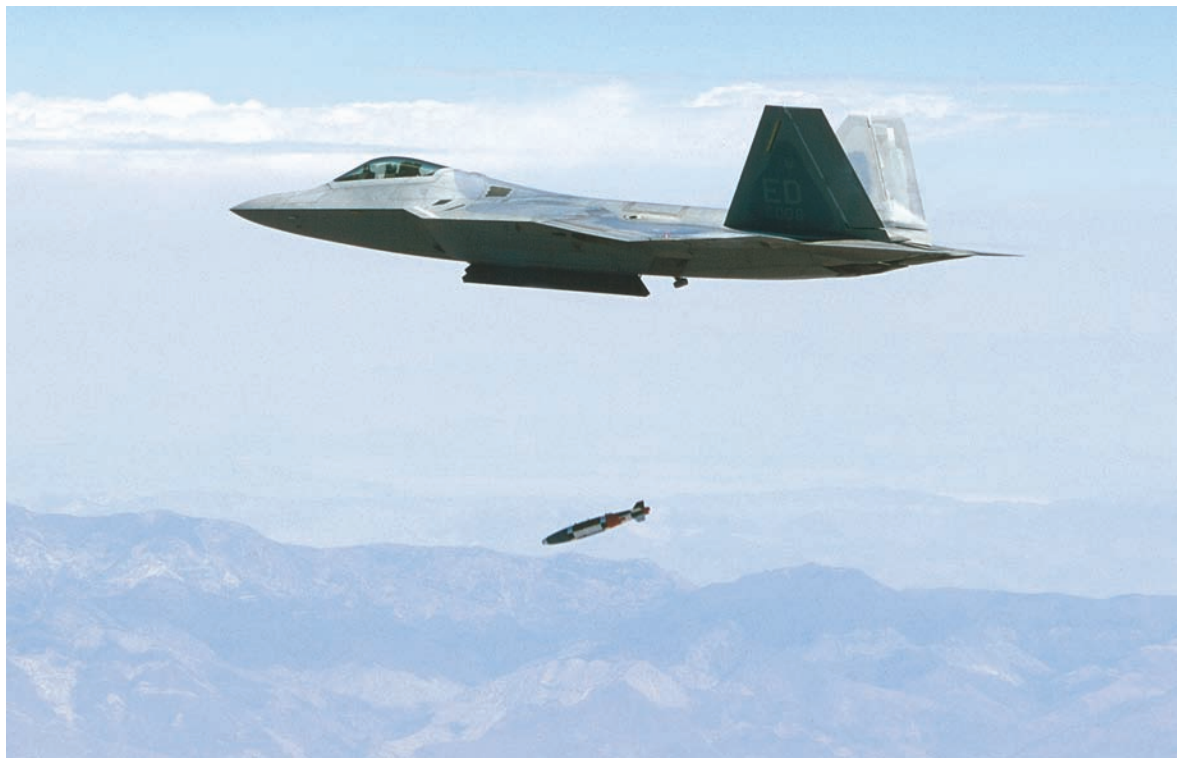
First supersonic release of the 1,000 lb GBU-32 Joint Direct Attack Munition GPS aided smart bomb from an F/A-22A Raptor over the Mojave test range in July, 2005. (US Air Force)
