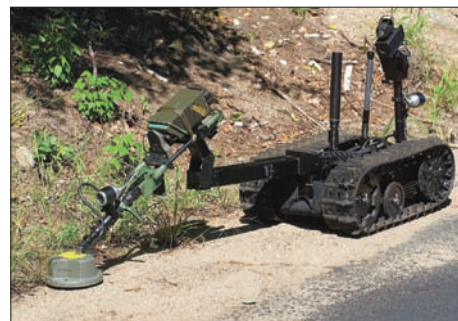
Talon IED detector robot sensing the roadside for munitions.
