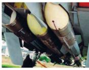
acquiring a 5 square metre target at 21.5 NMI. Range performance varies with the flight profile, from 80 NMI for a direct shot, to a maximum of 215 NMI for a cruise glide profile. In 1994 a trial round killed a target at
