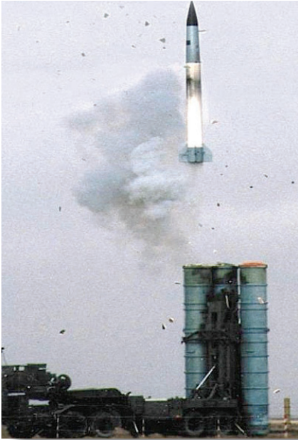
SA-20 missile launch. Late build SA-20B systems share technology extensively with the later SA-21, this including almost identical 54K6E2 and 55K6E command post vehicles, and 5P85TE2 and 5P85TM towed TELs, using identical BZKT 6 x 6 high mobility tractors.
