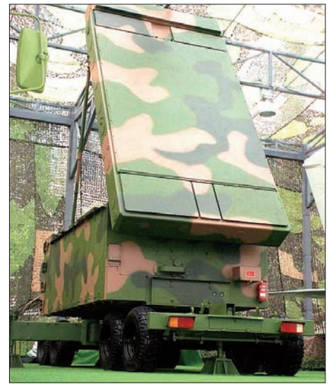
The Chinese H-200 radar is likely used in a hybridization upgrade of the SA-2 Guideline.
