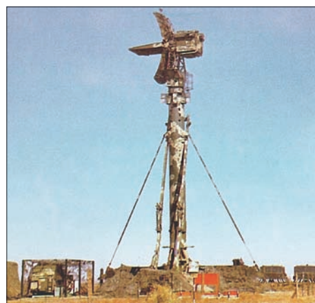
40V6M masts are available to extend low altitude coverage in SA-10/20 and SA-21 systems.
