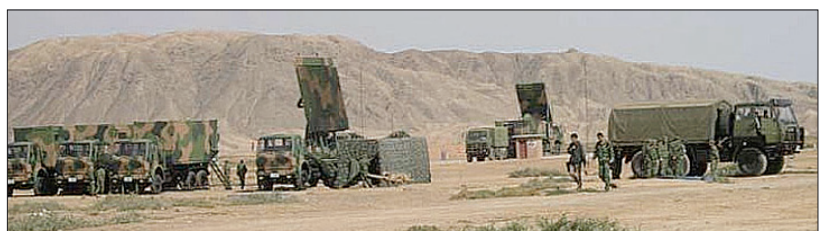
Chinese HQ-9 / FD-2000 SAM system components. Batteries are supported by modern Type 120, Type 305A and Type 305B high mobility radars on licenced Mercedes-Benz trucks. The Type 305A phased array is modelled on the new Thales Groundmaster.
