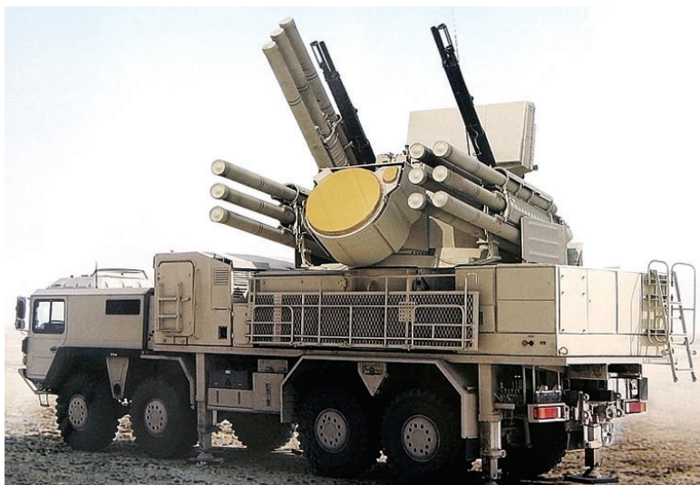
SA-22 system exported to the UAE. Like the SA-15D, it is intended primarily for defeat of the HARM/AARGM, JASSM and smart bombs during terminal flight.
