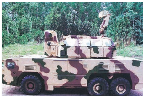
Late model SA-15D Gauntlet on hardened MZKT-6922 chassis. The SA-15D is intended primarily for defeat of the HARM/AARGM, JASSM and smart bombs during terminal flight.
