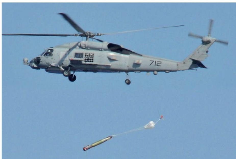
*Drop of a Mk-46 lightweight ASW torpedo from a Seahawk ASW helicopter.*
