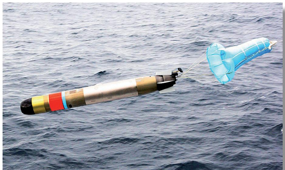
*The MU90 is an electrically powered lightweight torpedo.*
