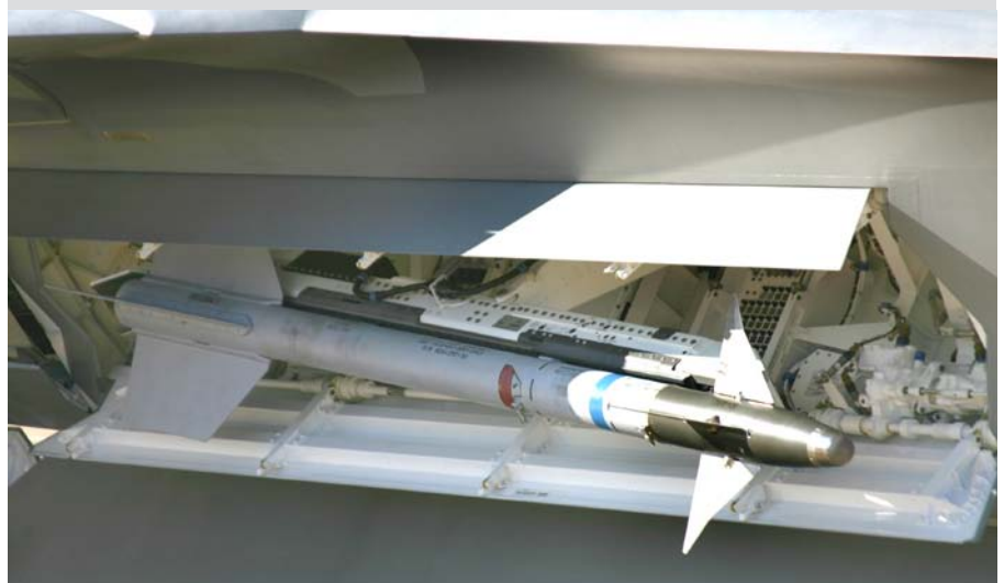
The starboard intake weapons bay of a Langley based F-22 showing an AIM-9M training round on its retractable rail. The latest generation AIM-9X is expected to be introduced onto the Raptor from mid 2007. (Andrew McLaughlin)
