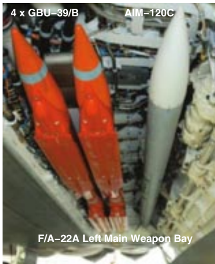
The new 285lb Boeing GBU-39/B is the weapon of choice for stealthy strikes on battlefield, urban or other smaller targets. The JSF carries eight weapons internally, with growth up to 20 – the F/A-22A also carries eight (depicted), with growth to 12 weapons.
