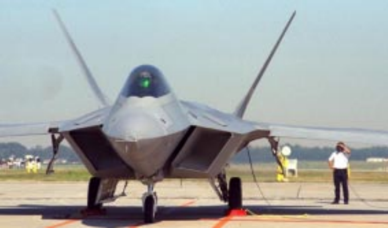
Both the F/A-22A and JSF use similar planform alignment and stealth shaping rules, reflecting a common design heritage. In the critical forward sector, the much more refined design of the F/A-22A is evident especially in the edge aligned inlet configuration and cleaner chining. The F/A-22A scatters into a smaller number of lobes over a much wider frequency band, reflecting its all aspect 'wideband' stealth requirement. (USAF & LM)
