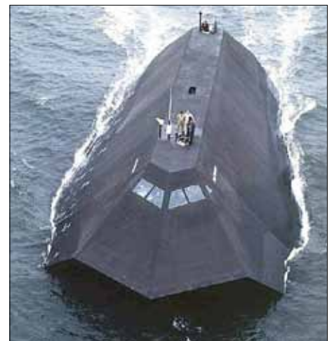
The US Navy Sea Shadow demonstrator proved the viability of faceted hull shaping. A period anecdote was that to find this vessel on radar, the operator needed to look for a black spot on the screen comprising the radar shadow of the vessel, where wavelop clutter was hidden by the invisible ship.
