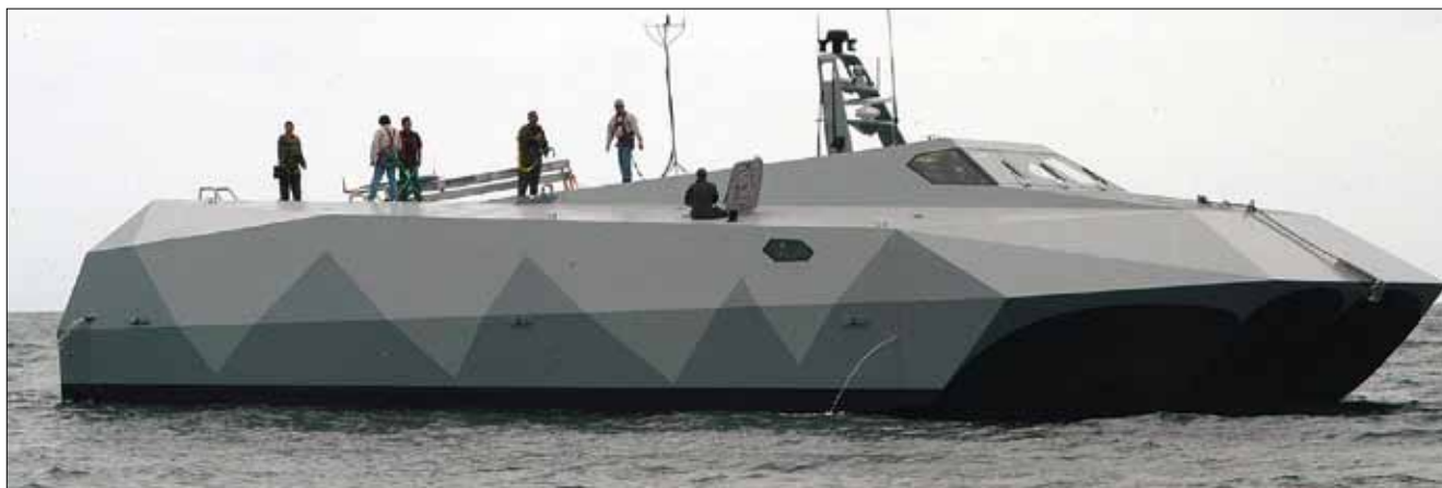
The carbonfibre "M-Hull" M-80 Stiletto demonstrator was developed as a platform for deploying SEAL special forces. It combines very good hull faceting with an "M-hull" configuration to provide 50 - 60 knot speeds.
