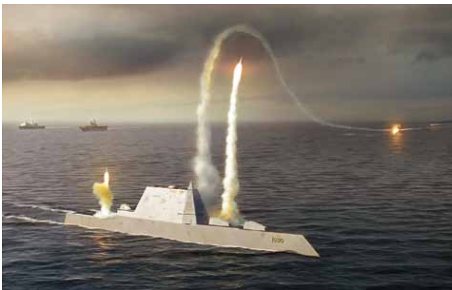
The USS Zumwalt class destroyer sets the benchmark for stealth shaping in future surface combatants.
