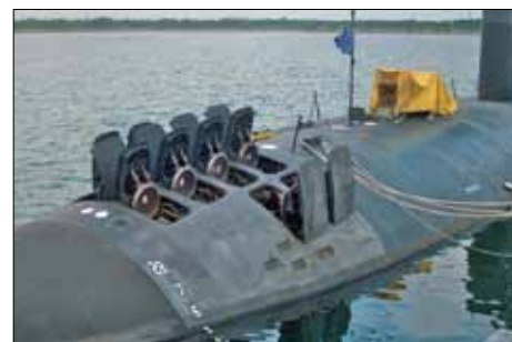
USS Santa Fe displaying its twelve open vertical launch tubes for SLCMs. Later Virginia class boats use a six round launcher arrangement adapted from the Ohio SSGN design, with two large doors.
