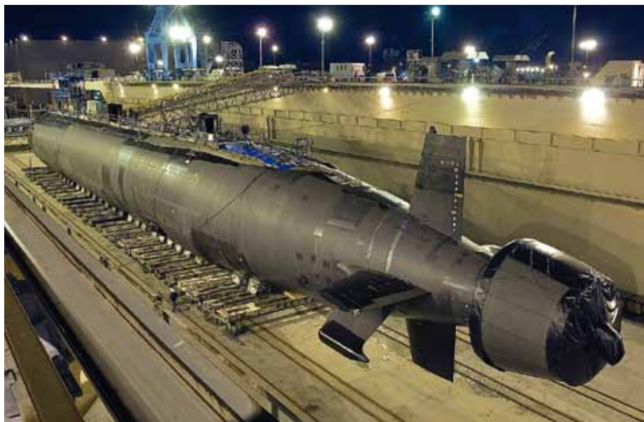
Virginia class SSN USS Washington displaying its propulsor system. Prof Ross Babbage recently proposed that Australia acquire this state of the art boat.
