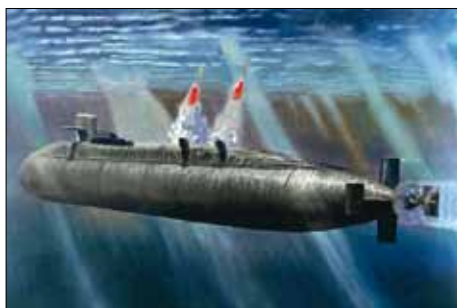
The Ohio class SSGN is a conversion from an SSBN, armed with up to 154 Tomahawk cruise missiles, in six round launchers which are inserted into former Trident SLBM tubes.
