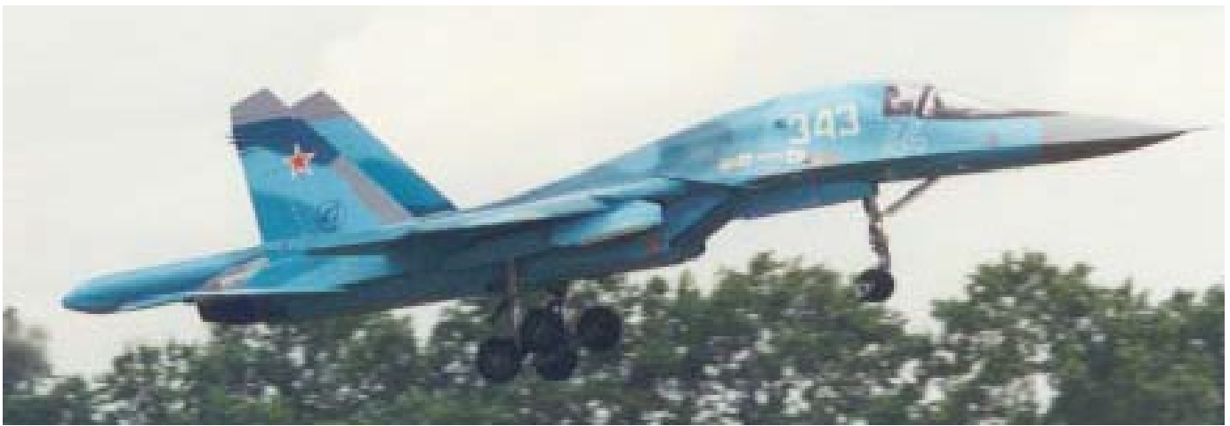
This image captures the unique fuselage hump design, enlarged spine and tail 'stinger', and tandem mains to effect.
