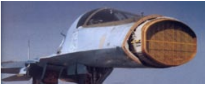
The B004 multimode phased array attack radar is the most advanced strike radar ever designed for a Russian combat aircraft. Unlike the N011M/BARS, the B004 is an optimised bomber radar, similar in many capabilities to the APQ-164 in the B-1B, and sharing the same generation of antenna technology. This image shows a prototype radar, and also exposes the fixed geometry intakes unique to the Su-32/34 series (Sukhoi).
