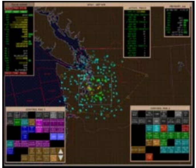
The new design consoles in the Wedgetail build on three decades of experience with the E-3 AWACS, but use COTS hardware and software to provide best possible capability at affordable costs. Demonstrators used Unix hosting hardware and X11/Motif windowing software (Boeing).
