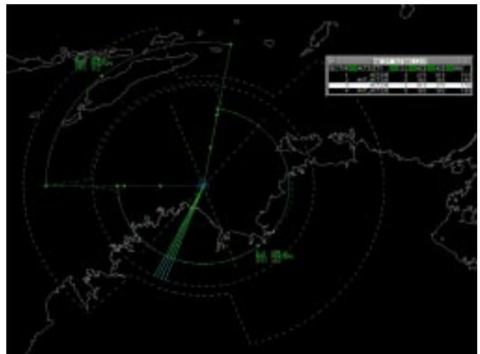
The Wedgetail's software intensive system will permit the use of a wide range of flexible, graphics intensive synthetic display formats, which can fuse radar, ESM, datalink and digital mapping outputs. These demonstrator displays illustrate the style of presentation to be used. This technology permits rapid growth to incorporate offboard data sources such as UAVs, satellites and ground based databases (Boeing).
