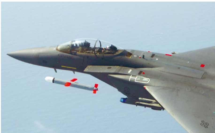
Late model Block IV Tactical Tomahawk and F-15E chase plane during trials.
