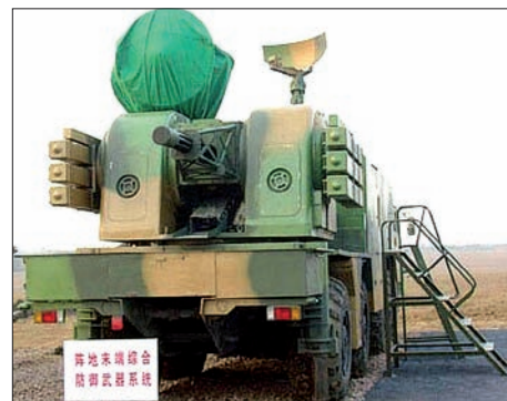
The Chinese LD-2000 SPAAGM, base on the Dutch 30 mm Goalkeeper, has considerable but yet to be fully developed potential as a C-RAM/C-PGM system. The LD-2000 has been integrated with a cloned Chinese TPQ-36 Counter Battery Radar.
