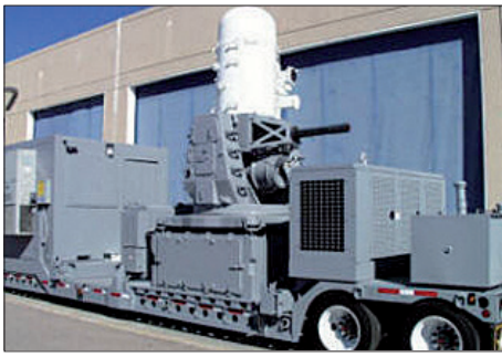
The US Army's new C-RAM Phalanx combines the existing naval CIWS system with existing CBR radar.
