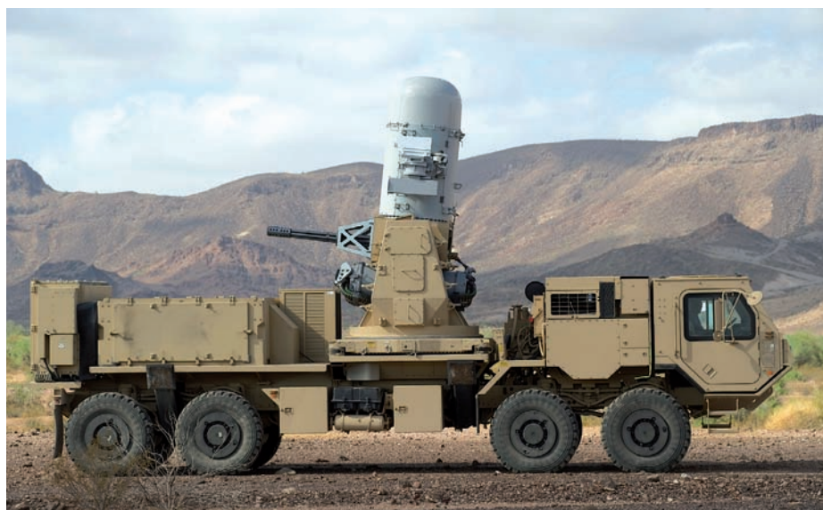
C-RAM Phalanx is a land based derivative of the naval CIWS.
