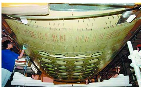
Ventral aft fuselage exhaust ports for the COIL laser.
