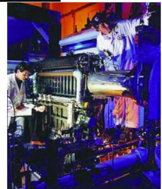
A single stage of the COIL laser.
