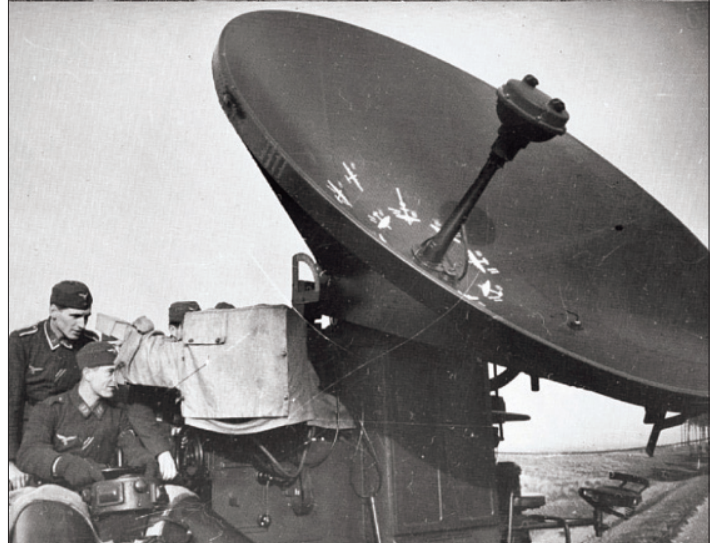
Precision tracking for intercepts was provided by the ubiquitous Telefunken FuSE 65 Würzburg-Riese, with Flak gunlaying provided by the smaller FuSE 62 Würzburg.
