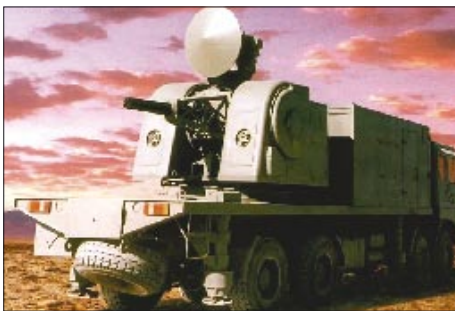
The LD-2000 Gatling gun is capable of killing smart munitions as they close on their targets.
