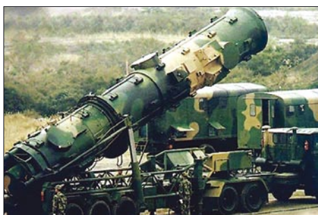
The DF-21 IRBM is derived from the JL-1 SLBM, and is the basis of the PLA ASAT and ASBM weapons.
