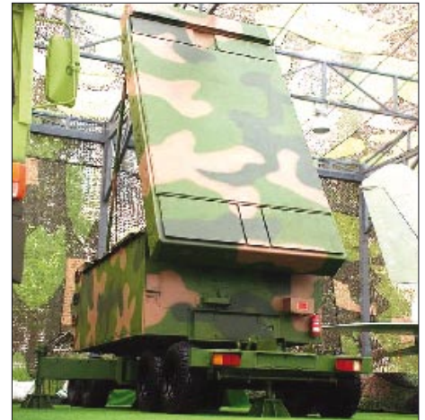
The indigenous H-200 phased array engagement radar.
