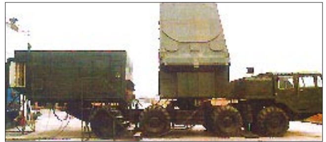
The HT-233 is a derivative of the Russian 30N6 series and is a jam resistant agile beam engagement radar.
