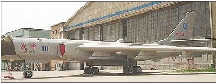
The H-6K is a new turboprop powered variant capable of hitting targets beyond 2,000 NMI range, with up to seven large cruise missiles.
