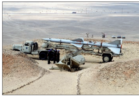
Egyptian SA-2 battery components, an SM-90 launcher, V-75 missile and SNRA-75 Fan Song radar.
