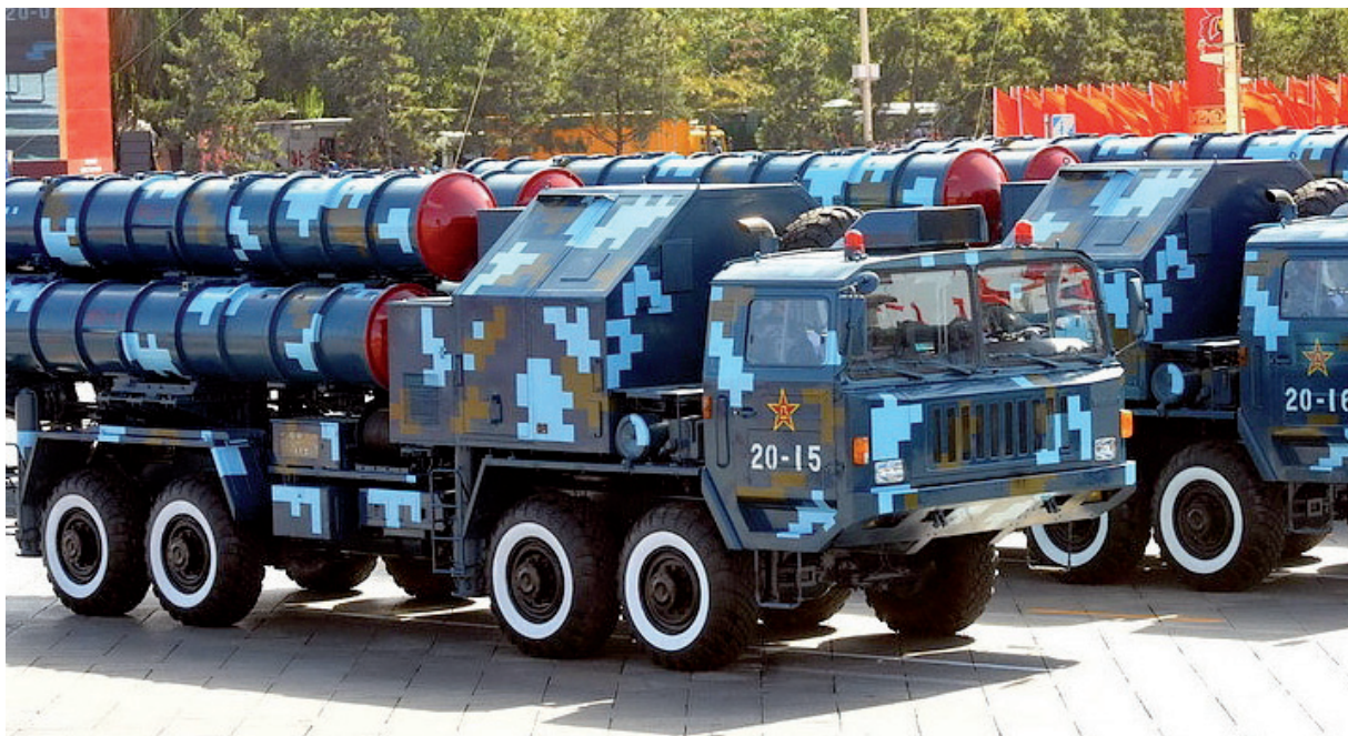
Modern SAMs like this Chinese HQ-9 system have none of the vulnerabilities of the SAMs defeated in the Middle East, and employ highly automated digital fire control systems and radars. They are direct equivalents to the US MIM-104 Patriot, but much more mobile and thus survivable in the face of air attack.
