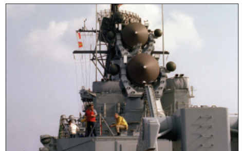
Mechanically steered X-band illuminators to support missile shots have until recently been a common design feature in air defence destroyers and cruisers.
